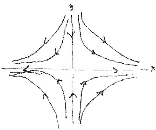
$$\textcircled{3} \quad a) \quad \bar{x}' = \underbrace{\begin{pmatrix} 1 & 2 \\ 2 & 1 \end{pmatrix}}_A \bar{x}, \quad \bar{x}(0) = \begin{pmatrix} 0 \\ 2 \end{pmatrix}$$
