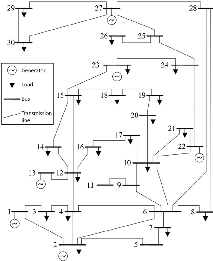
Figure 2.1: Schematic of the IEEE 30-bus test system representing its generators, loads, busses and transmission lines.
