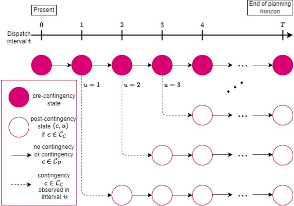
Figure 4.1: Illustration of the dispatch following a contingency under corrective security.
