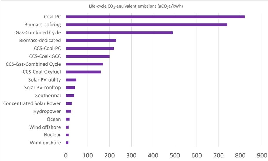
Figure 1.1: Median values of life-cycle greenhouse gas emissions for various generation sources.
