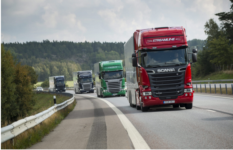
Figure 1.2: Four-vehicle platoon driving over an uphill stretch. (Photo provided by courtesy of Scania AB.)
