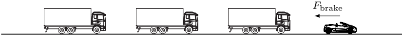
(a) Automatic braking of a platoon due to the interference of an external vehicle.
