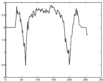
Figure 1.21: Selected scale levels along a central horizontal cross-section through the wedding-cake type random dot stereo pair in figure 1.20. Observe that distinct minima are obtained at the two discontinuities in the disparity field.
