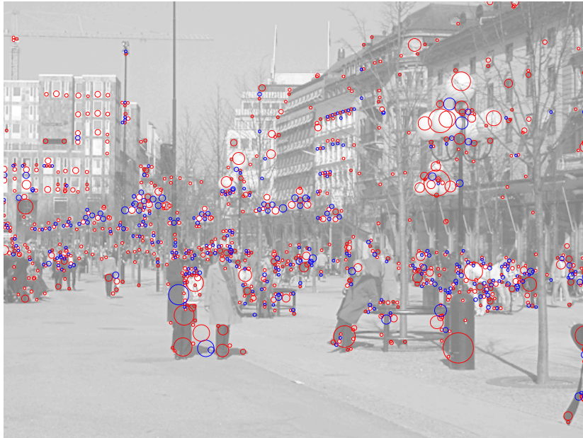
scale-space extrema of the determinant of the Hessian \det \mathcal{H}_{norm} L
