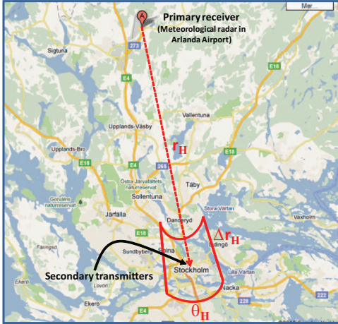
Fig. 2. An application of the hot zone model to Stockholm area. The map is captured from http://www.eniro.se/ .
