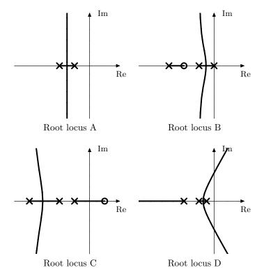
Figure 3.19b. Starting points (K=0) are marked  $\times$ , and end points  $(K\to\infty)$  are marked  $\circ$ . All diagrams have equal scaling.
