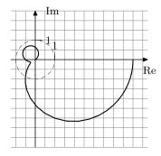
Figure 9.16b. Nyquist curve of the loop gain.
