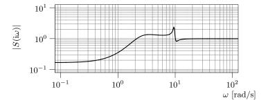
Figure 9.16c. Gain curve of the sensitivity function.
