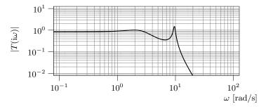
Figure 9.16d. Gain curve of the complementary sensitivity function.
