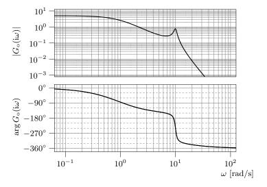
Figure 9.16a. Bode plot of the loop gain.
