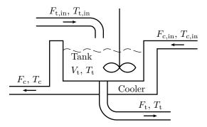
Figure 3.30a. Process consisting of a tank and a cooler. Input flows have a "in" subscript, while outputs have no such subscript since they are also the same as the quantities found inside the tank or cooler.
