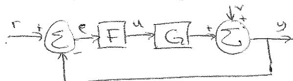
$$\begin{cases} Y = V + GU \\ U = FE \\ E = R - Y \end{cases} \Rightarrow Y = V + GF(R - Y) \Rightarrow Y = \underbrace{\frac{1}{1+GF}}_{G_{vy}=S} V + \underbrace{\frac{GF}{1+GF}}_{\text{R}} R$$
