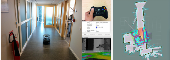
Fig. 4: The human-in-the-loop experiment setup, where the robot is controlled by both its autonomous controller and the human inputs.
