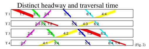
It is easy to see that for comparable total times the number of trains that can be scheduled with JSS on an identical network is significantly lower. It is possible to achieve a schedule similar to the second one using a network with a larger number of (shorter) tracks but then the size of the scheduling problem increases accordingly.
