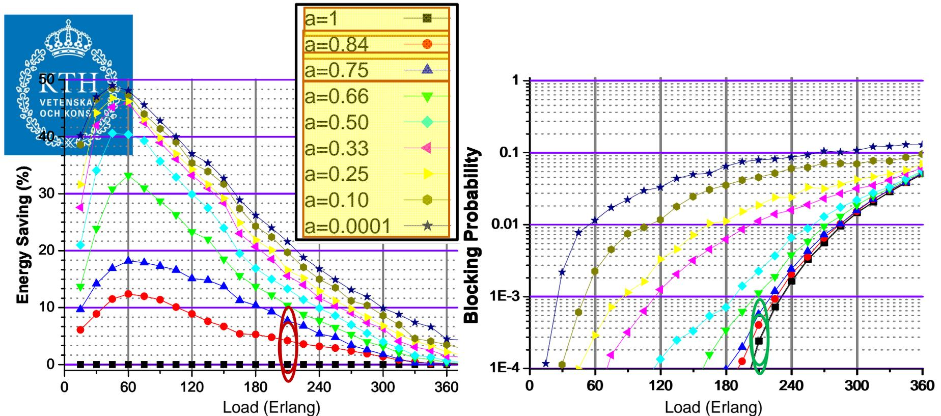
"Cost" of the link: use  $C_{link} = a_{link} * E_{link}$ , where  $0 \leq a_{link} \leq 1$ ,  $E_{link}$  = energy consumption of a link; not in use  $C_{link} = E_{link}$
