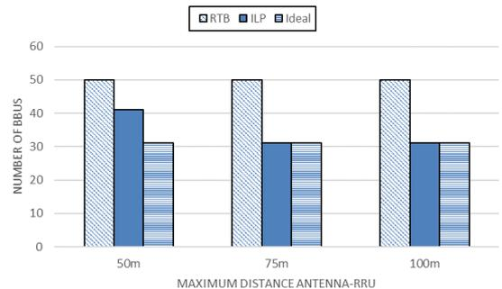
Fig. 4. Number of BBUs as a function of the maximum distance between antenna and RRU.
