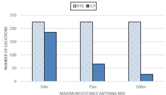
Fig. 5. Number of locations that needs to be activated as a function of the maximum distance between antenna and RRU.
