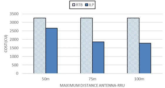
Fig. 6. Total cost of the network as a function of the maximum distance between antenna and RRU.
