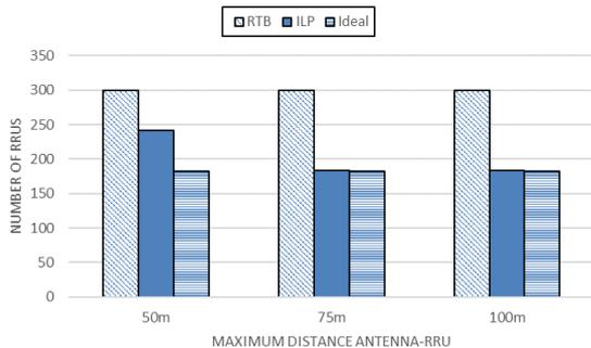
Fig. 3. Number of RRUs as a function of the maximum distance between antenna and RRU.
