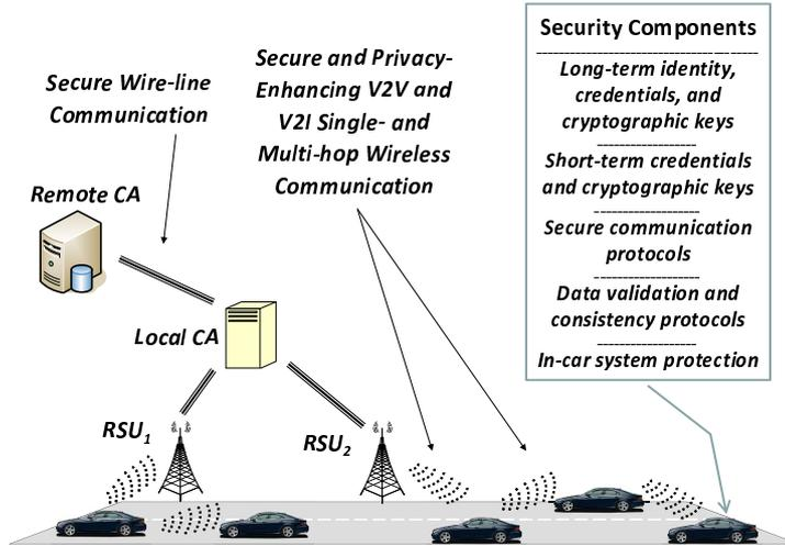
Figure 1: Abstract View of a Secure Vehicular Communication System.
