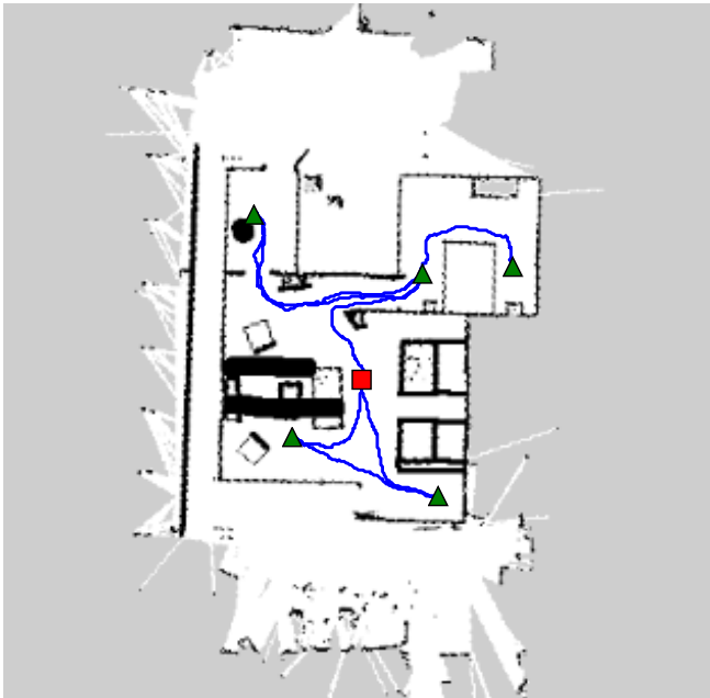
Figure 4: Path traveled by the SocRob@Home robot during a run of the navigation functionality benchmark. The squares represent the initial position while the triangles denote the given waypoints.
