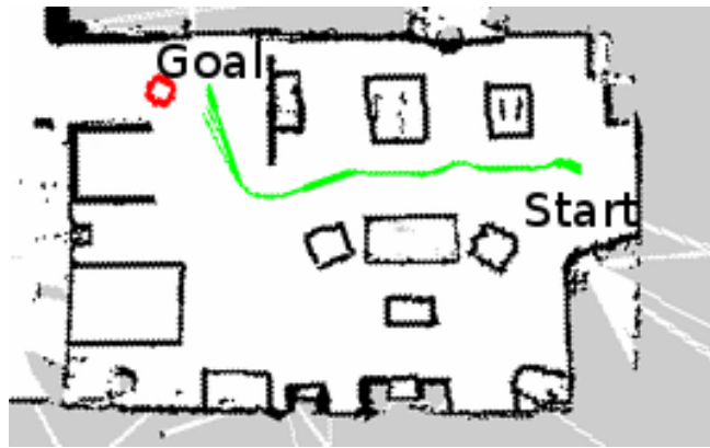
(d) Results for Experiment 4. Green lines show robot's paths to reach the person for object hand over. Person location in each run are shown in red circles.
