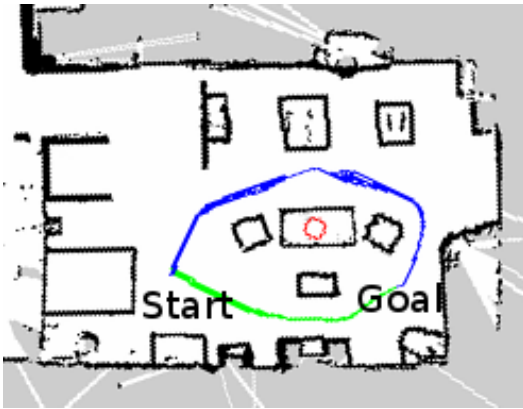
(c) Results for Experiment 3. Green lines show robot's final paths computed with TV off. Blue lines show the final robot's paths with TV on. Red circles identify person location.
