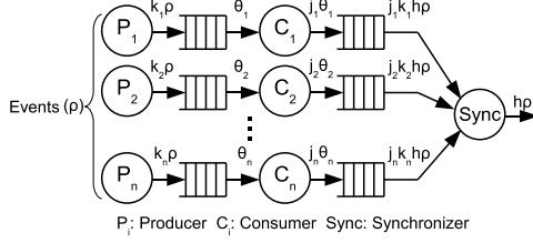
Fig. 1. Static SDF model for multi-streaming applications
