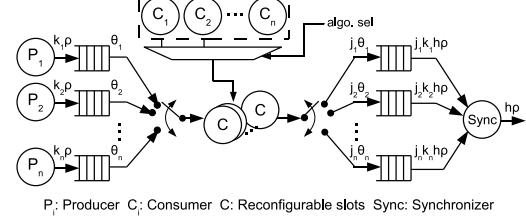
Fig. 2. Adaptive SDF model for multi-streaming applications
