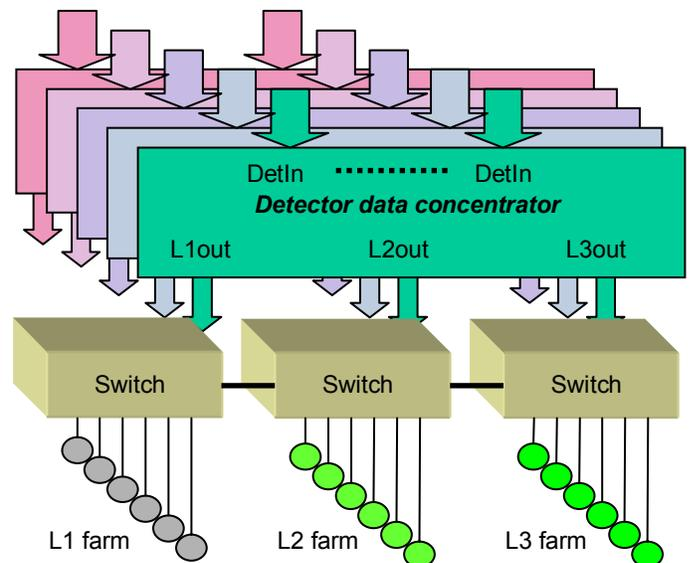
Fig. 2 Schematic overview of the PANDA data acquisition does not employ fixed hardware based triggers but features a continuously sampling system where the various subsystems are synchronized with a precision time stamp distribution
