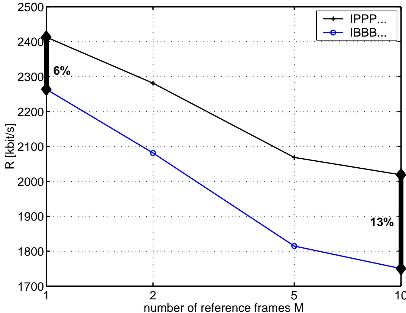
Avg. bit-rate at 35 dB PSNR for the CIF sequence *Mobile & Calendar*, 30 fps
