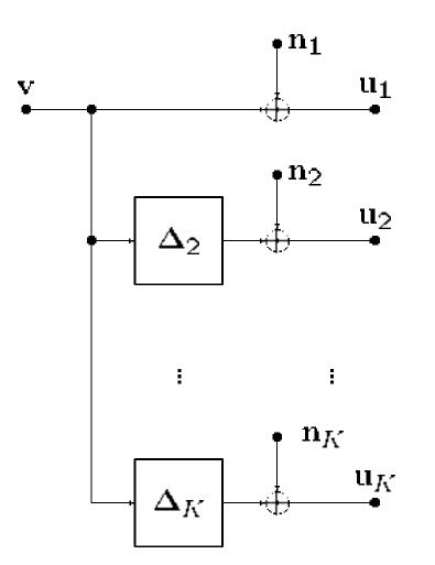
Model for coding with motioncompensated lifted wavelets [Flierl & Girod, 2003]
