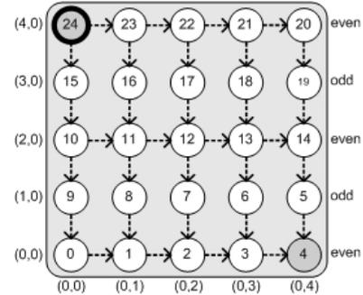
Fig. 3. All of the possible minimal paths from the source node 24 to the destination node 4 of the proposed model for unicast messages.
