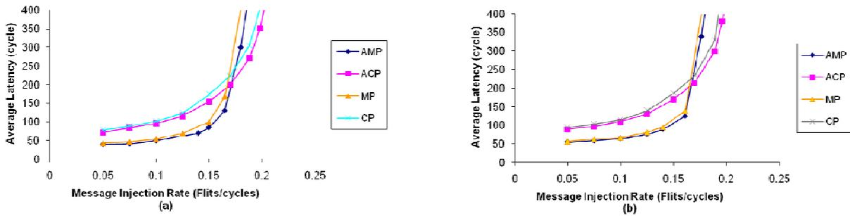
Fig. 7. Performance with different loads in  $8 \times 8$  2D-mesh with (a) 10 destinations, (b) 25 destinations under mixed traffic (20% multicast and 80% unicast). Unicast traffic is based on the hotspot traffic model with a single hotspot node (4, 4), and  $h=10\%$ .
