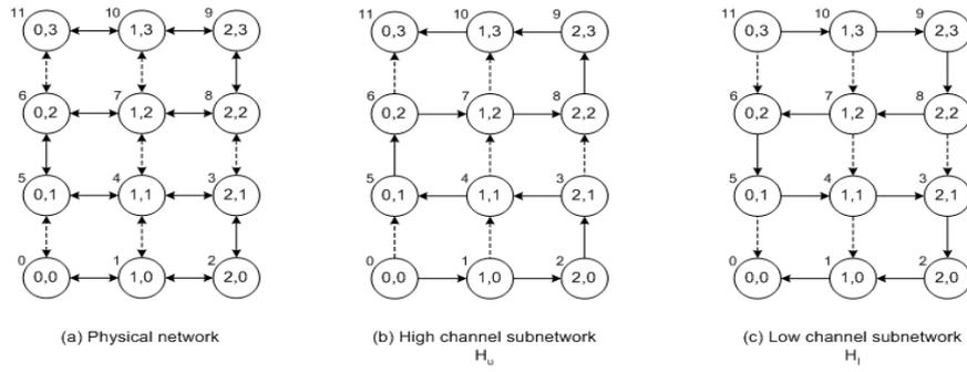
Fig. 1. (a) A  $3 \times 4$  mesh physical network with the label assignment and the corresponding (b) high channel and (c) low channel networks. The solid lines indicate the Hamiltonian path and dashed lines indicate the links that could be used to reduce path length in routing.
