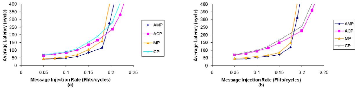
Fig. 6. Performance with different loads in  $8 \times 8$  2D-mesh with (a) 10 destinations, (b) 25 destinations under mixed traffic (20% multicast and 80% unicast). Unicast traffic is based on the uniform traffic model.
