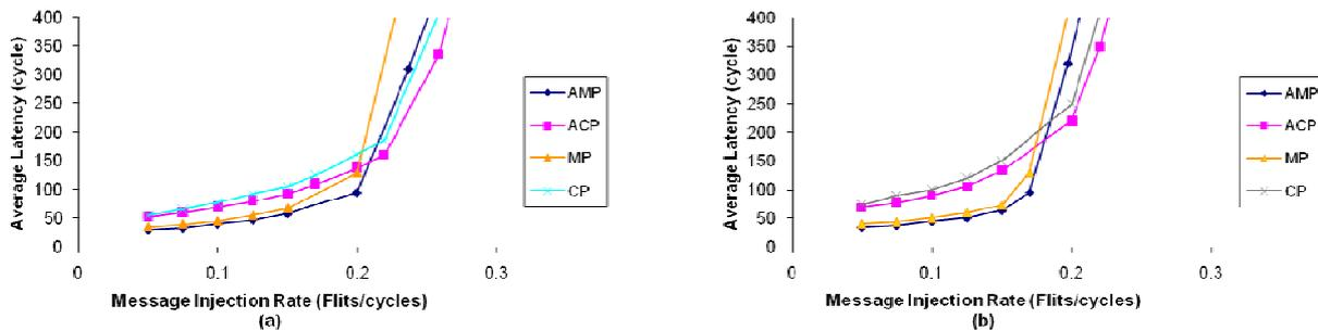
Fig. 5. Performance with different loads in 8×8 2D-mesh with (a) 10 destinations, (b) 25 destinations.
