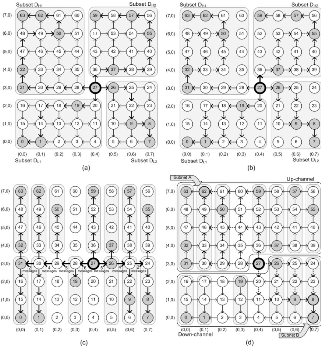
Fig. 2. Examples of (a) Multi-path (MP), (b) Adaptive Multi-Path (AMP), (c) Column-Path (CP), and (d) Adaptive Column-Path (ACP) multicast routings from the node 27 (to subsets A, and B for column path example). The unused links are not indicated.
