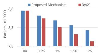
Fig. 10 Fault-tolerant capability under Bit-Reversal Traffic
