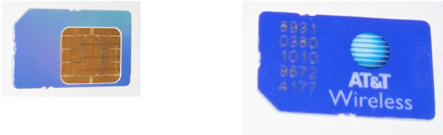
Figure 25: SIM card showing contacts on the left and the IMSI on the right
