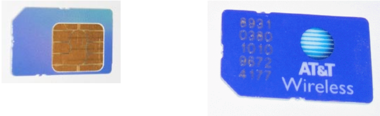
Figure 22: SIM card showing contacts on the left and the IMSI on the right
