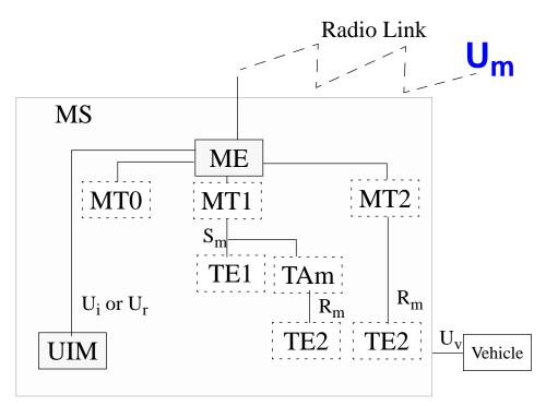
Figure 34: 3GPP2 Architecture (the mobile)
