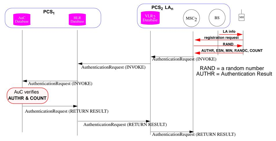
Figure 16: Mobile moves into a new Location Area (LA) at PCS<sub>2</sub>
