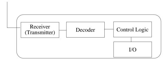
I/O can be a display, a beeper, keypad, audio input/output, vibrator, ....
