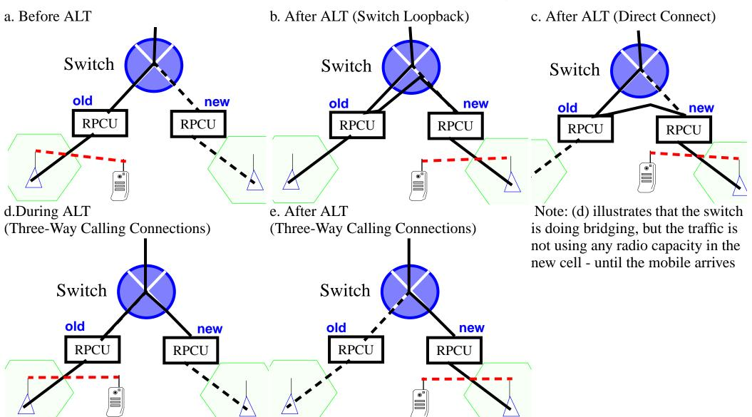
Maguire3 alternative inter-RPCU handoff methods (Switch Loopback, Direct Connection, Three-way Calling Connection): Netmaguire@it.kth.se 2004.03.17 Net-Mobile and Wireless Network Architectures
