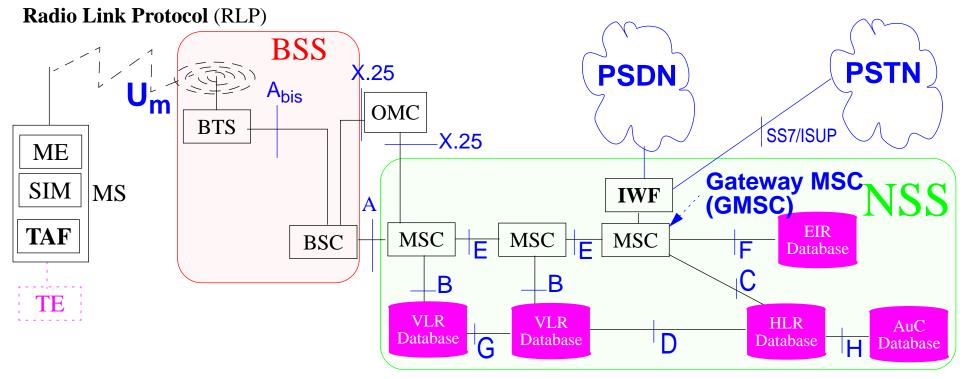
Figure 25: GSM/HSCSD Architecture
