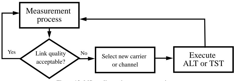
Figure 12: MS-quality maintenance processing
