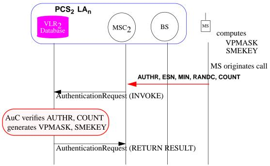
Figure 19: Mobile places a call in PCS<sub>2</sub> using sharing scheme
