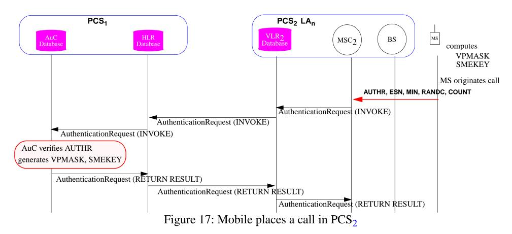
Because of SSD the AuC can generate the same Voice Privacy Mask (VPMASK) and Signaling Message Encryption Key (SMEKEY) as the mobile and passes this information to the operator of  $PSC_2$
