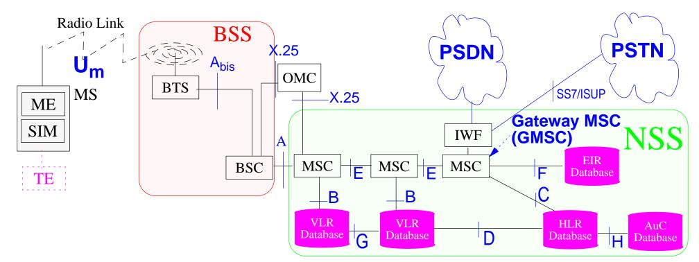
Figure 23: GSM Architecture
