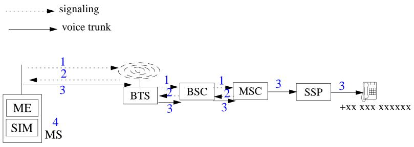
Figure 33: Handset-Based Prepaid call origination
