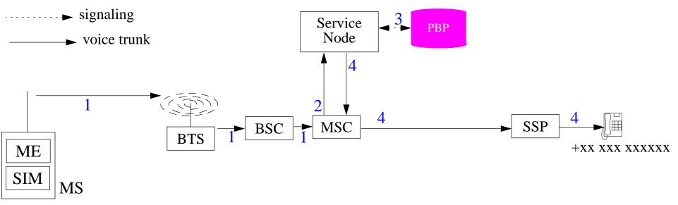
Figure 31: Service Node Prepaid call origination
