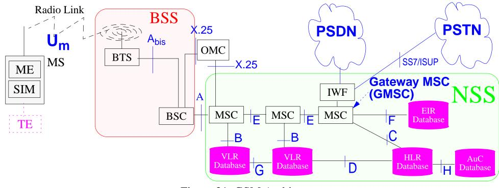
Figure 21: GSM Architecture
