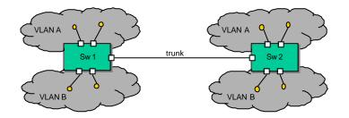
The figure above illustrates two VLAN switches (Sw 1 and Sw 2), two VLANs (A and B), and a VLAN trunk between the switches.
