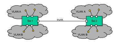
The figure above illustrates two VLAN switches (Sw 1 and Sw 2), two VLANs (A and B), and a VLAN trunk between the switches.
