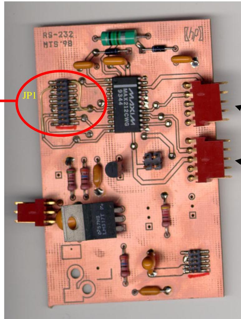
To modify the SmartBadge RS-232 buffer module to support ANGEL, you need to cut two traces and add two wires as shown above.
