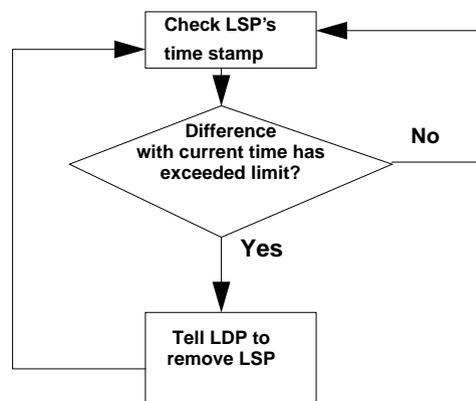
**Figure 28** - A background process checks for timed-out LSPs
