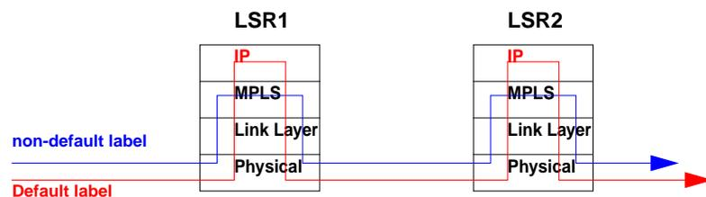
Figure 6 - Default-labeled packets are IP routed
