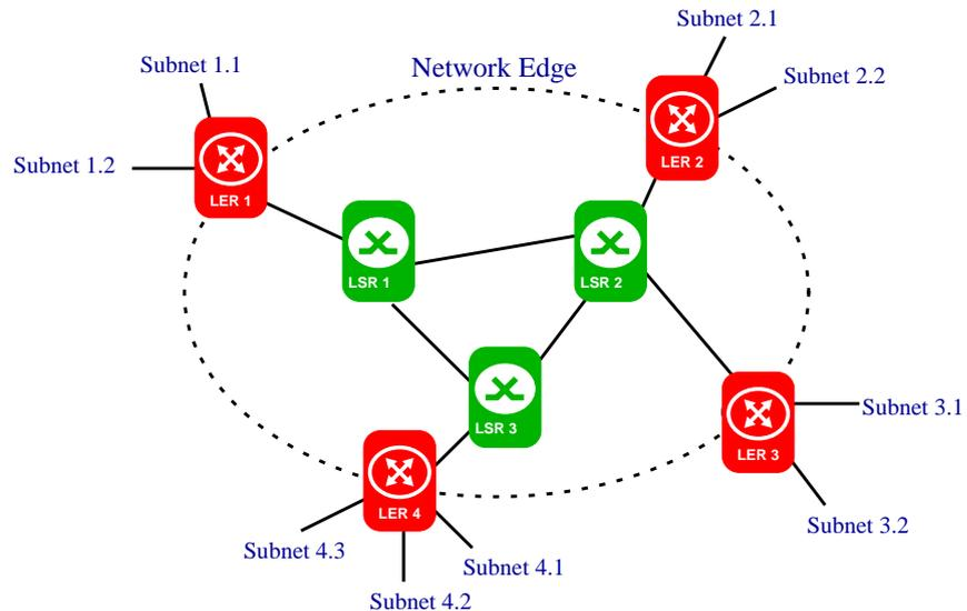
**Figure 2** - An example configuration of a MPLS network
