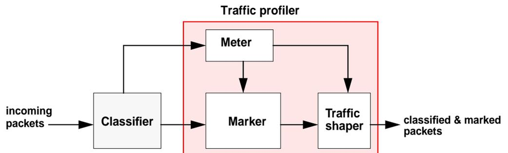
**Figure 13** - Architecture of a DiffServ boundary node
