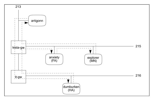
Figure 24. A ping from artigonn to the Mobile Node
