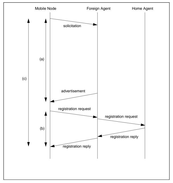
Figure 26. Sequence diagram for making a connection
