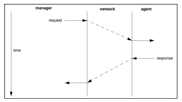
Figure 6. SNMP request-response interaction (based on [11] p. 243)
