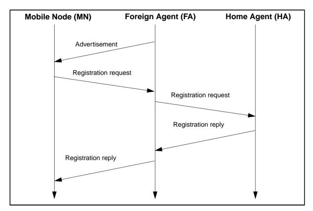
Figure 3. The messages sent when a Mobile Node register with a Home Agent through a Foreign Agent
