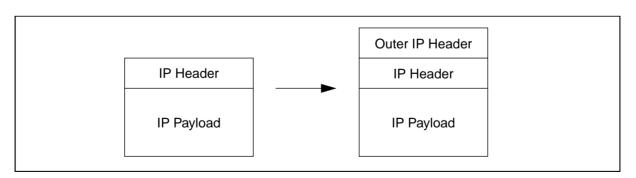
Figure 4. IP in IP encapsulation
