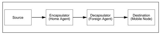
Figure 5. The general encapsulation case
