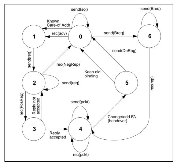
Here is the state diagram for the Mobile Node.
