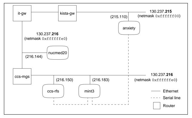
Figure 20. The subnetworks and the workstations in the lab
