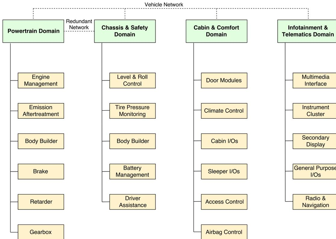
Figure 2.1: Example of a federated E/E architecture in commercial trucks
