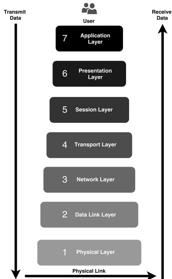
Figure 2.2: Open Systems Interconnect model of network layering
