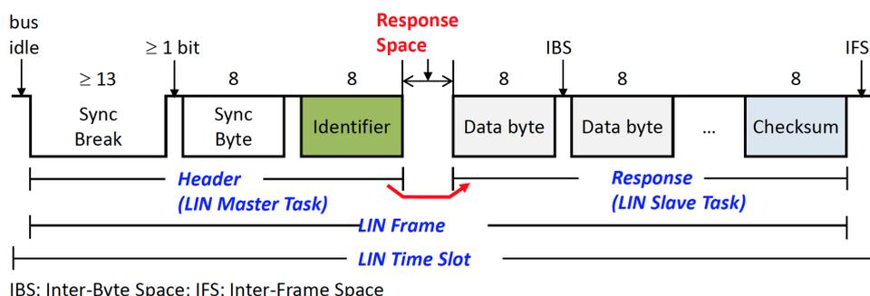
Figure 2.8: LIN frames transmission
