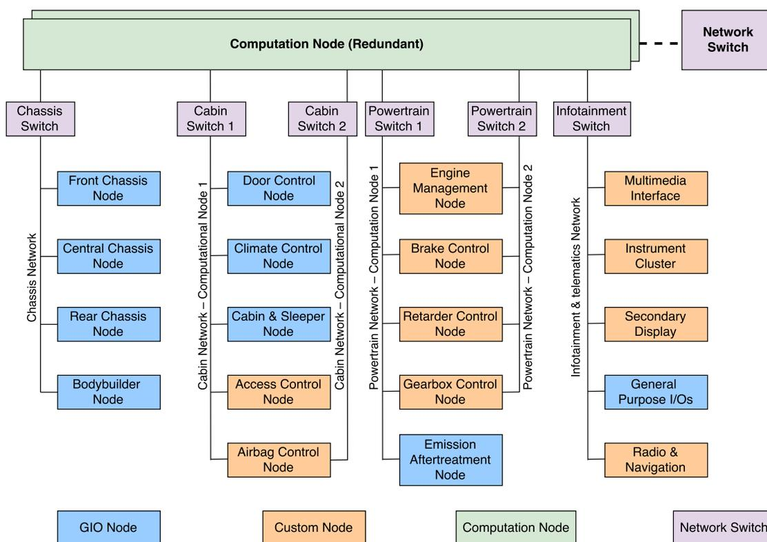
Figure 3.1: Example of the proposed partially redundant integrated E/E architecture for commercial trucks
