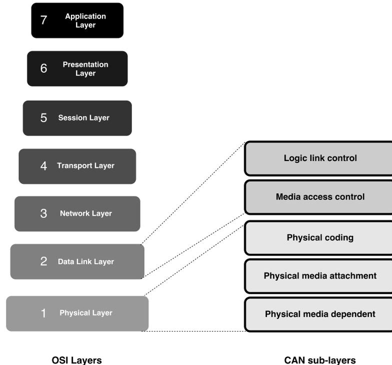
Figure 2.5: CAN sublayers with reference to ISO OSI model
