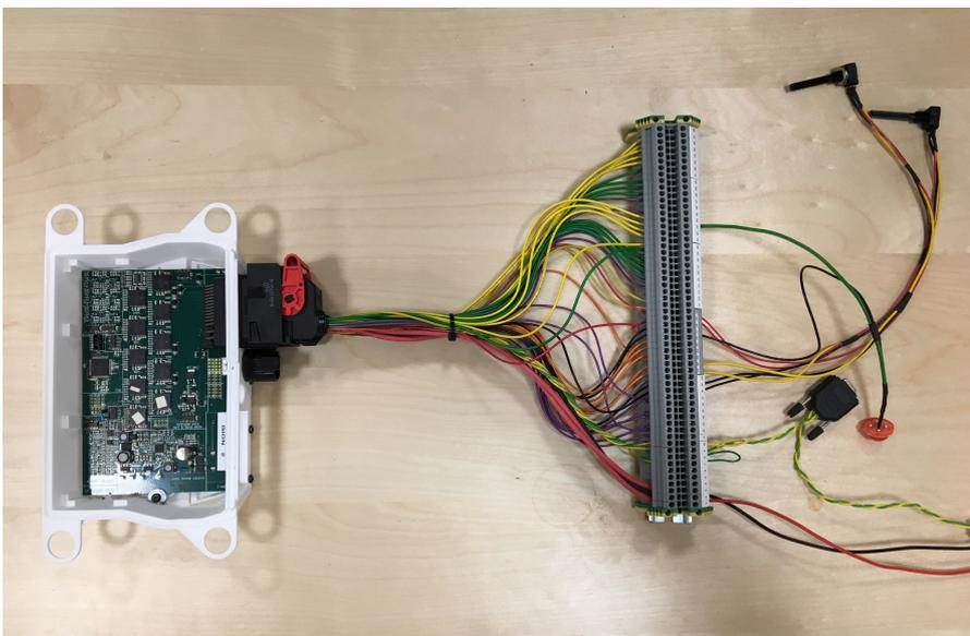
Figure 4.3: Generic I/O node prototype connected with the test rig
