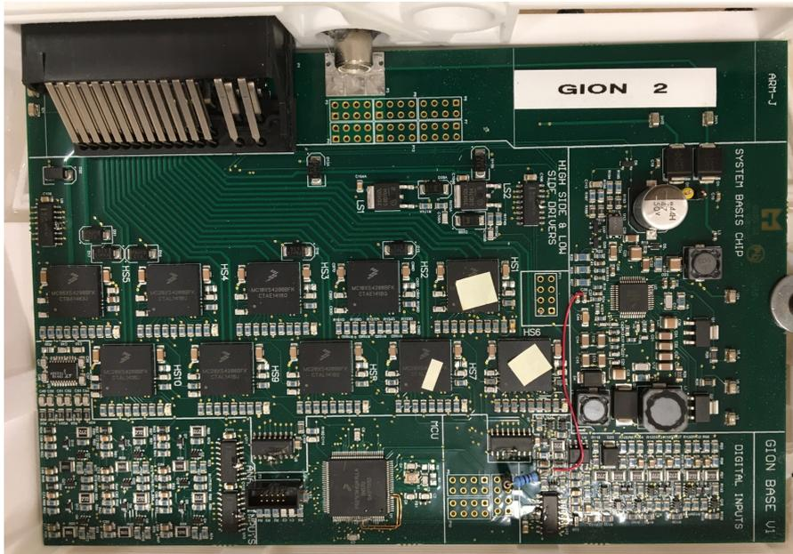
Figure 4.2: Generic I/O node prototype
