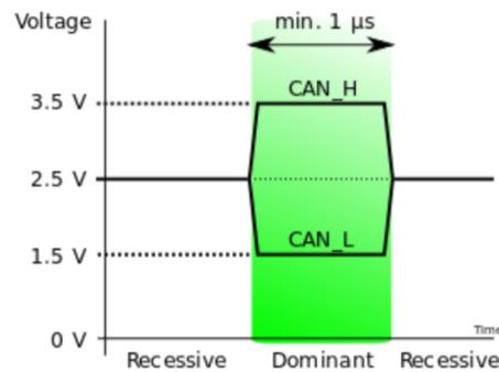
Figure 2.4: A CAN differential bus
