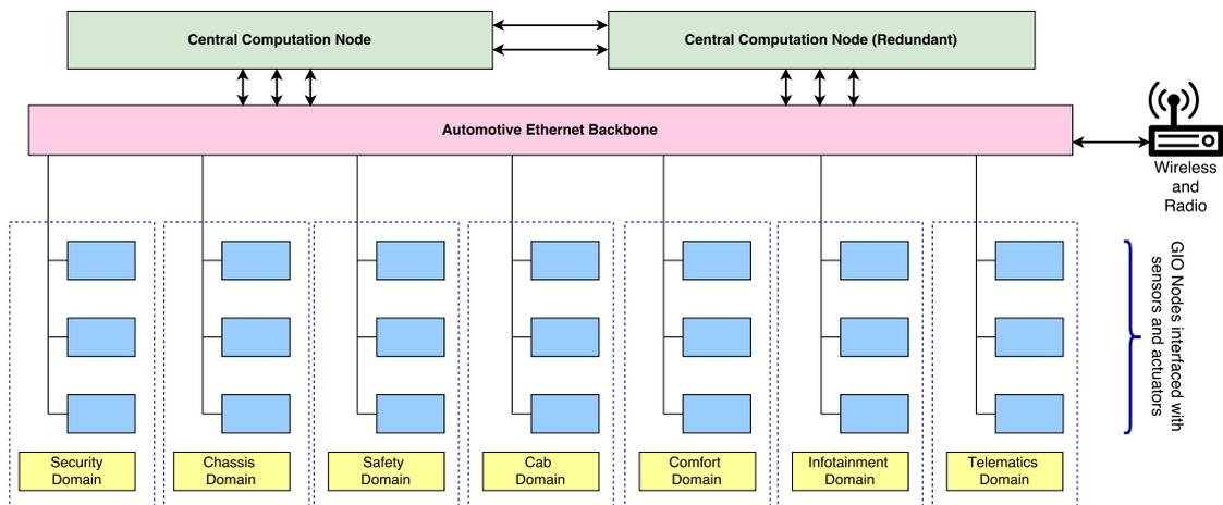
Figure 3.2: Future concept for next generation Integrated E/E Architecture
