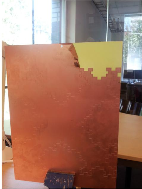
Figure 4.5: Process to remove the remaining copper from the copper clad board
