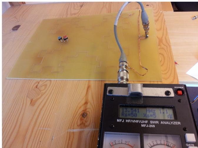
Figure 4.7: Matching for PCB Minkowski antenna 2 iterations
