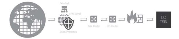
Figure 4-1: How a DDoS attack from the Internet is mitigated by the network outside of the data center (DC)
