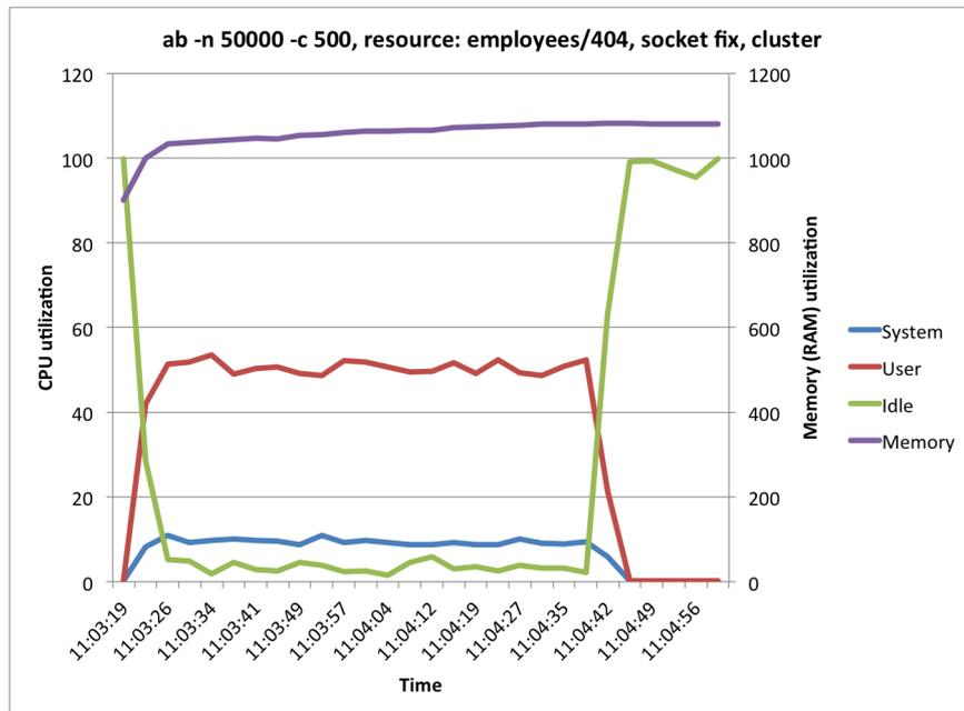
Figure 4.10: CPU and memory consumption during test
