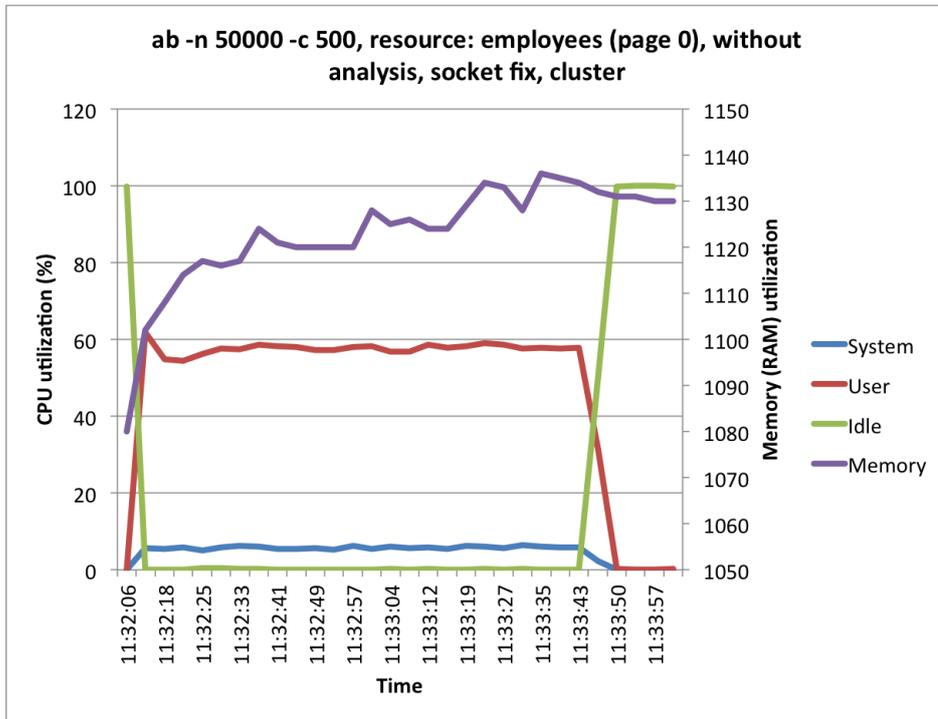
Figure 4.24: CPU and memory consumption during test
