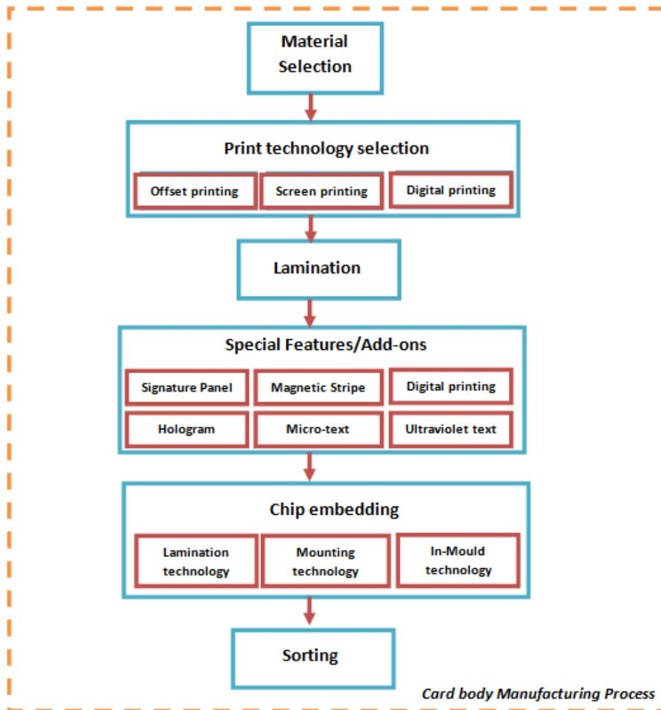
Figure 2.6: Card Body Manufacturing Process
