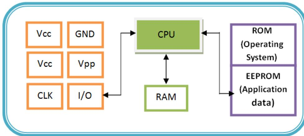
Figure 2.4: Architectural view of a microprocessor card [11]
