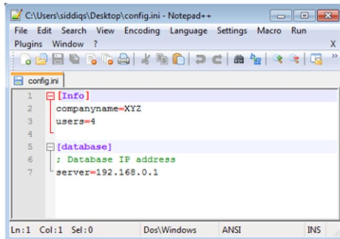
Figure 4.2: Config.ini file defines system initial parameters
