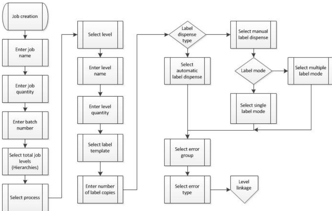
Figure 4.10: Flow chart: Job initial setup
