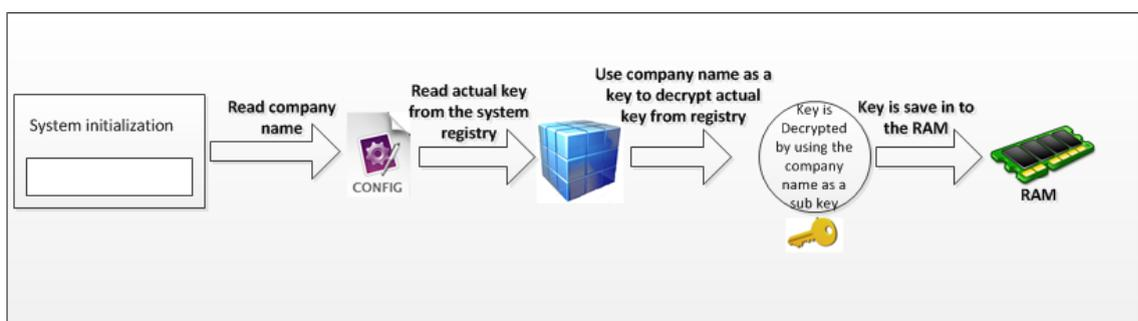
Figure 4.5: Encryption key reading procedure for data decryption
