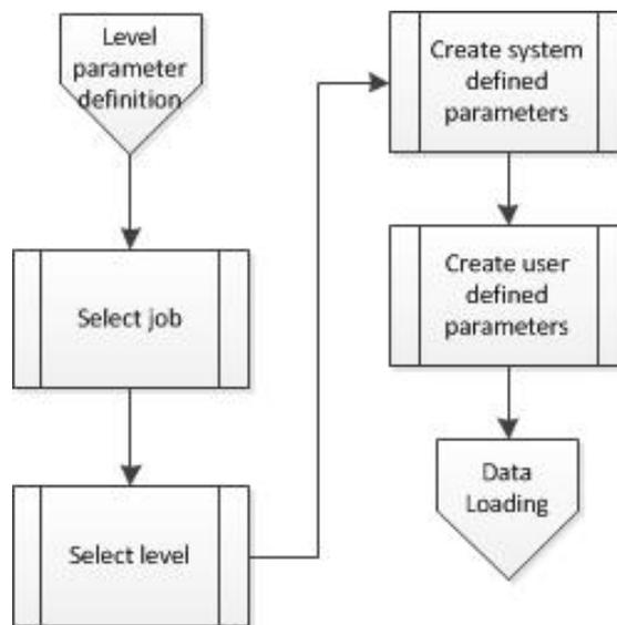
Figure 4.12: Flow chart: Level parameter definition
