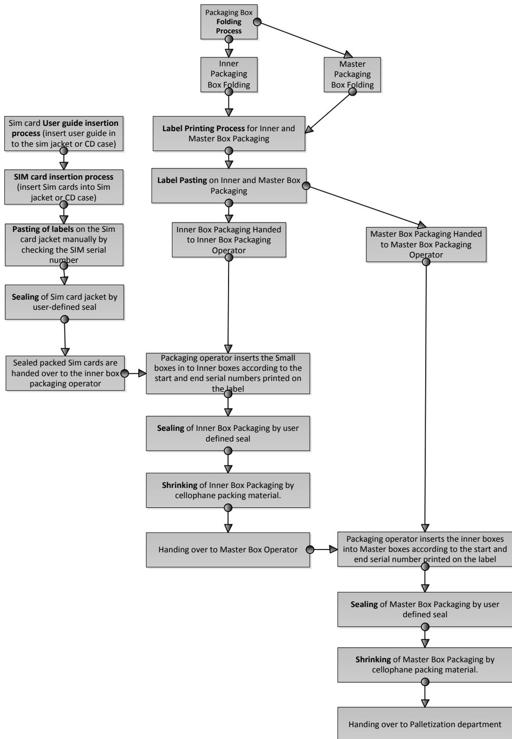
Figure 2.11: SIM cards packaging process flow diagram
