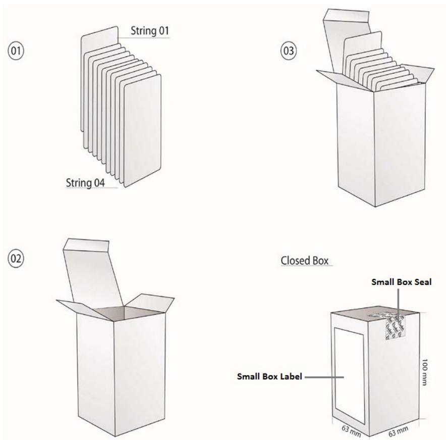
Figure 2.17: Small Box Scratch/Bank card Packaging
