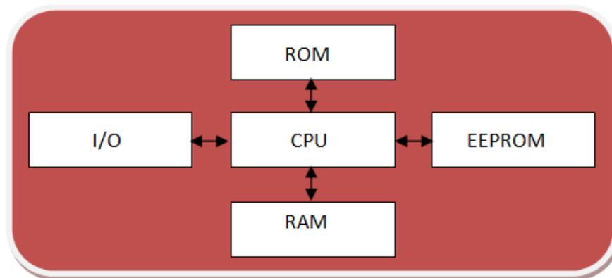
Figure 2.1: Smart card Architecture [36]
