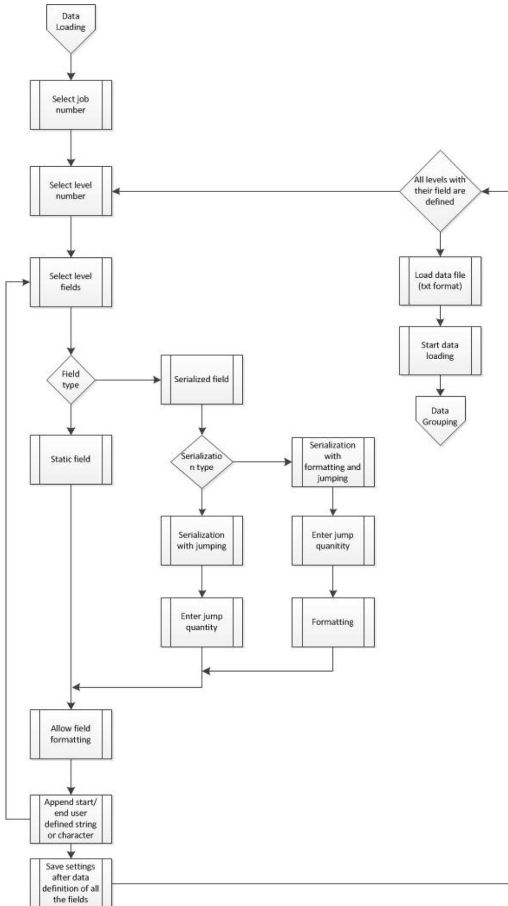
Figure 4.13: Flow chart: Data loading
