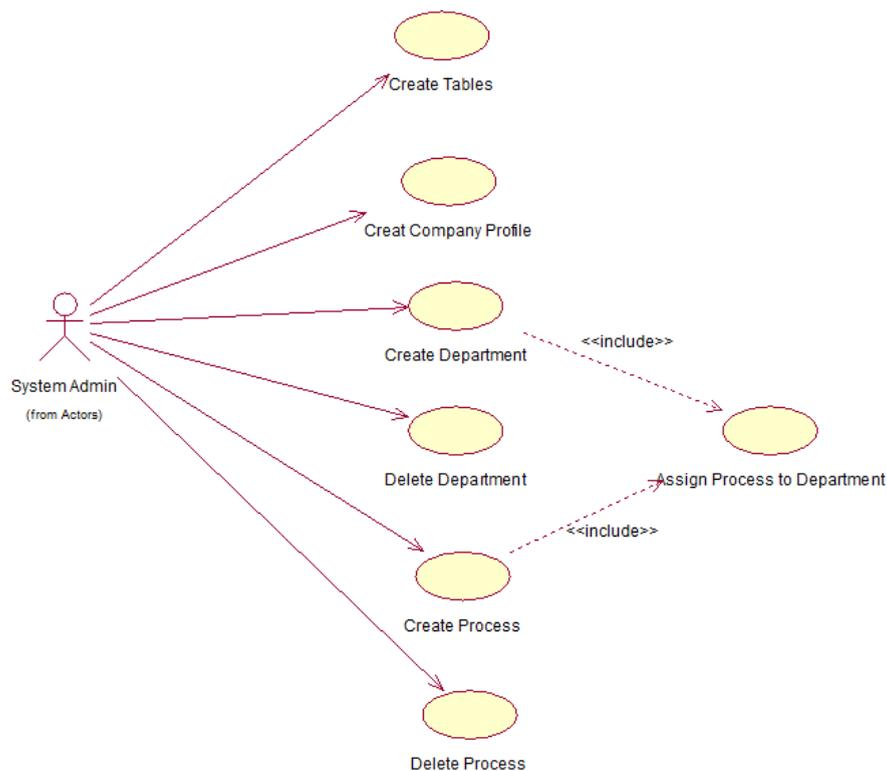
Figure 3.9: System initial setup use case diagram
