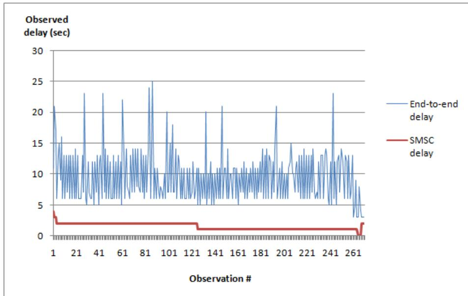
Figure 5.7: Comparison of end-to-end and SMSC delay
