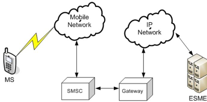
Figure 2.3: SMS-IP integration (adapted from [1])
