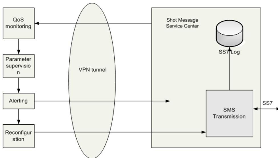
Figure 3.1: Framework for QoS monitoring[4]
