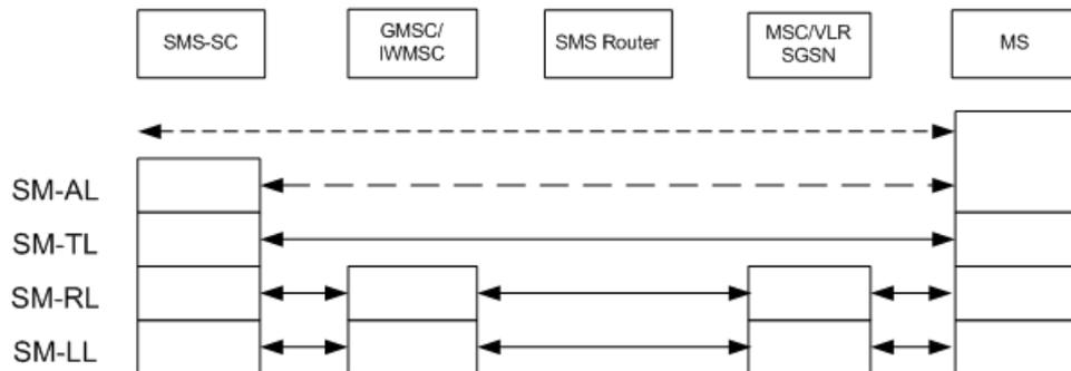
Figure 2.4: SMS protocol layers [3]
