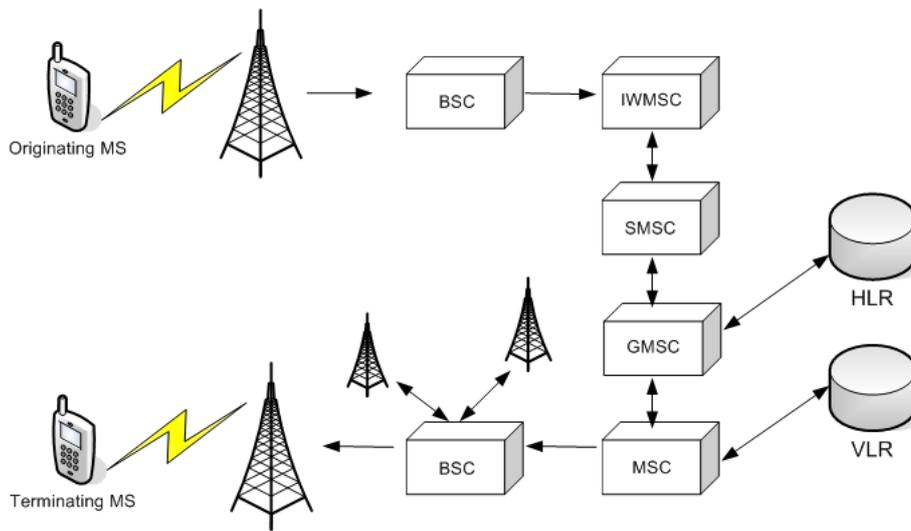
Figure 2.1: SMS architecture (adapted from [1])
