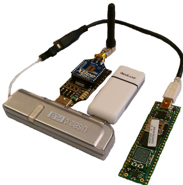
Figure 4.2: The hardware of the proxy prototype, where a Libelium Waspote Gateway and a 3G dongle are connected to a Gumstix Overo Earth through a USB hub.
