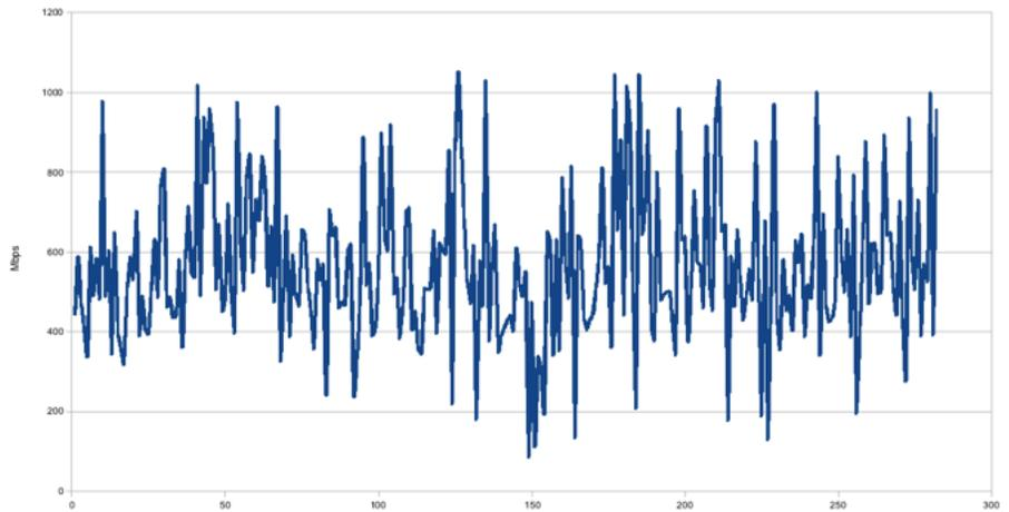
Figure 4.2: TCP bandwidth between two m1.small instances in Amazon EC2 (Source: [46])
