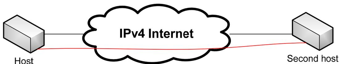
Figure 3: Semantic illustration of the 6in4 tunneling protocol (with the lower red line indicating the tunnel and the black lines indicating the actual network links)
