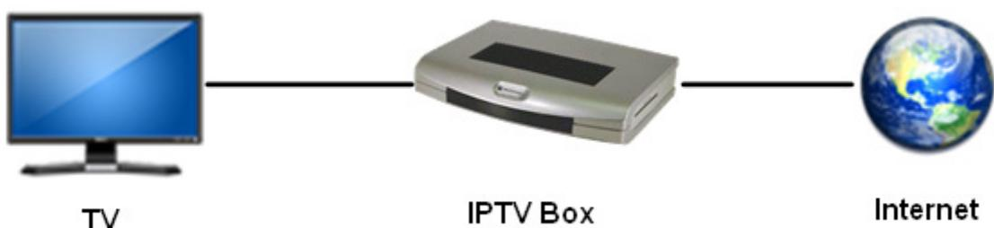
Figure 1-1: The basic components of IPTV
