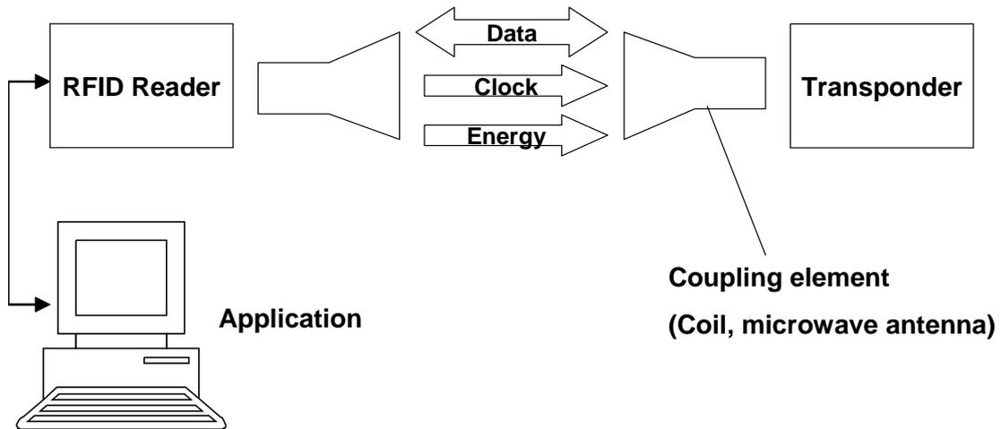
Figure A.1: Components of an RFID system (is adapted from [2])
