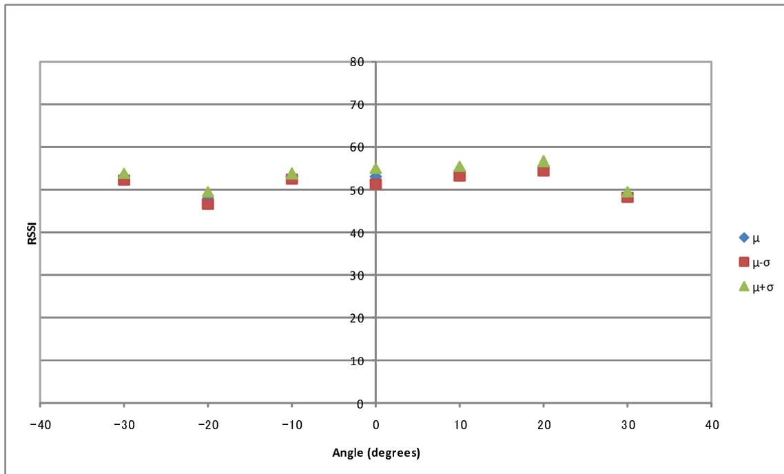
Figure 3.8: RSSI values at 10 degree steps with the antenna 3 meter from signal source
