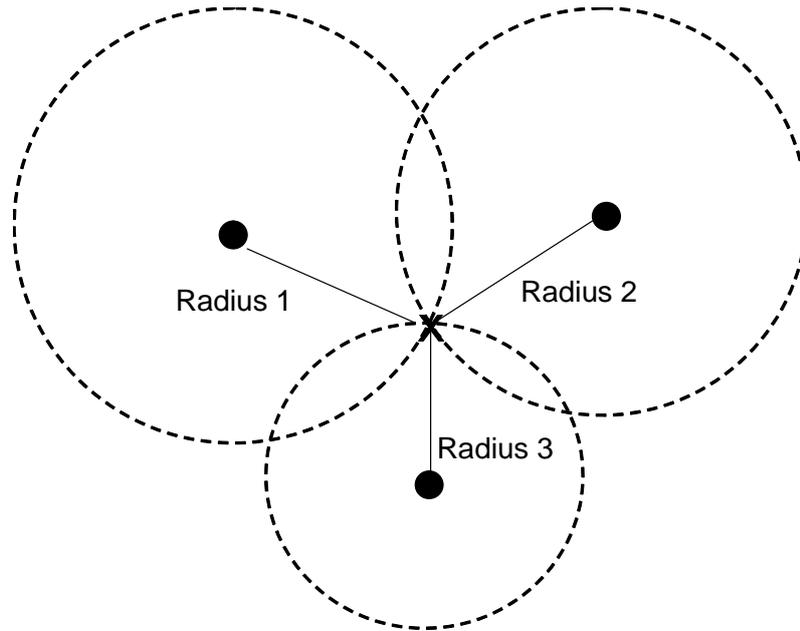
Figure 2.4: Determining 2D position by lateration
