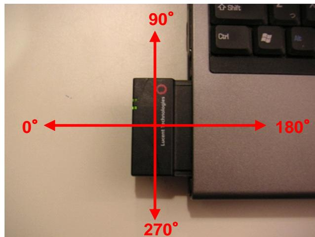
Figure 3.10: Orientation definition on signal source
