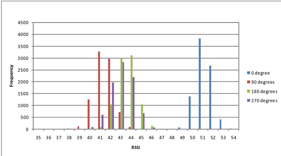
Figure 3.7: Histogram of RSSI values for four different antenna orientations
