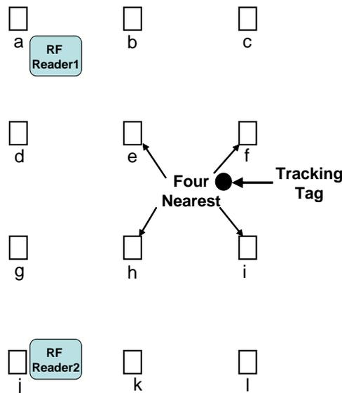
Figure 2.9: An example of a tracking tag and the nearest reference tags in LANDMARC
