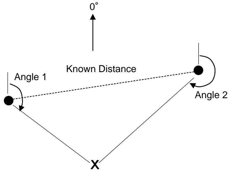
Figure 2.5: 2D angulation using two angles and the distance between two reference points
