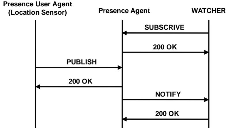
Figure 4.8: Message exchanged to update location from location sensor to WATCHER
