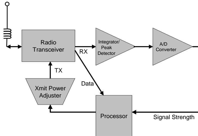
Figure 2.6: Hardware design of SpotON tag radio architecture
