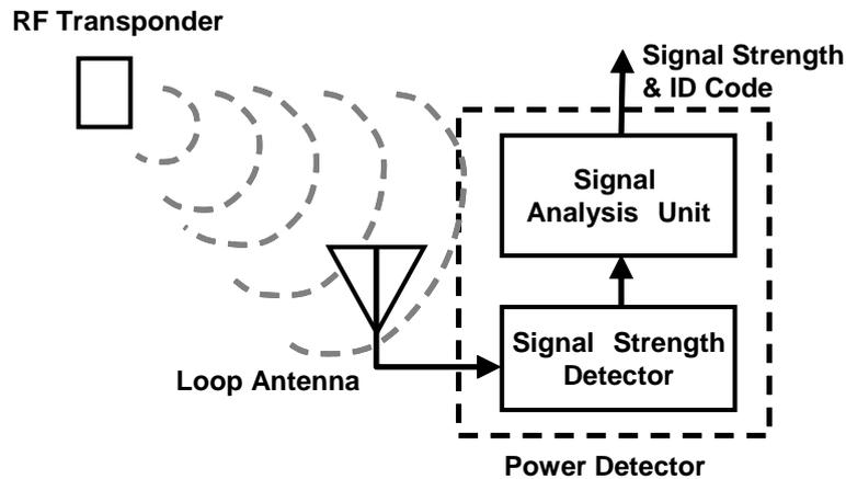
Figure 2.11: Schematic of loop antenna equipped with the signal strength detector
