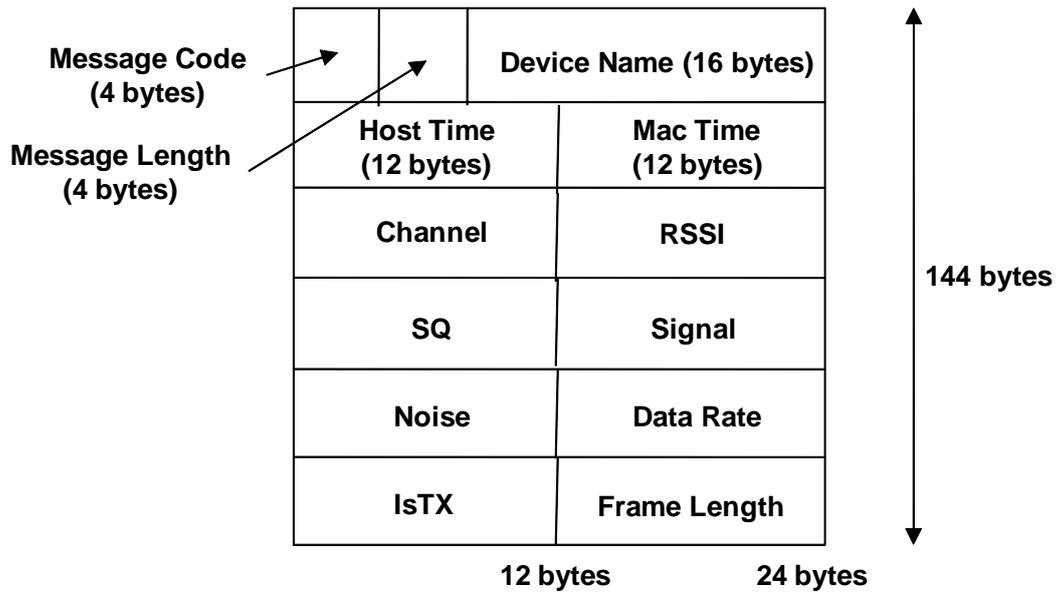
Figure 4.1: Prism monitoring header
