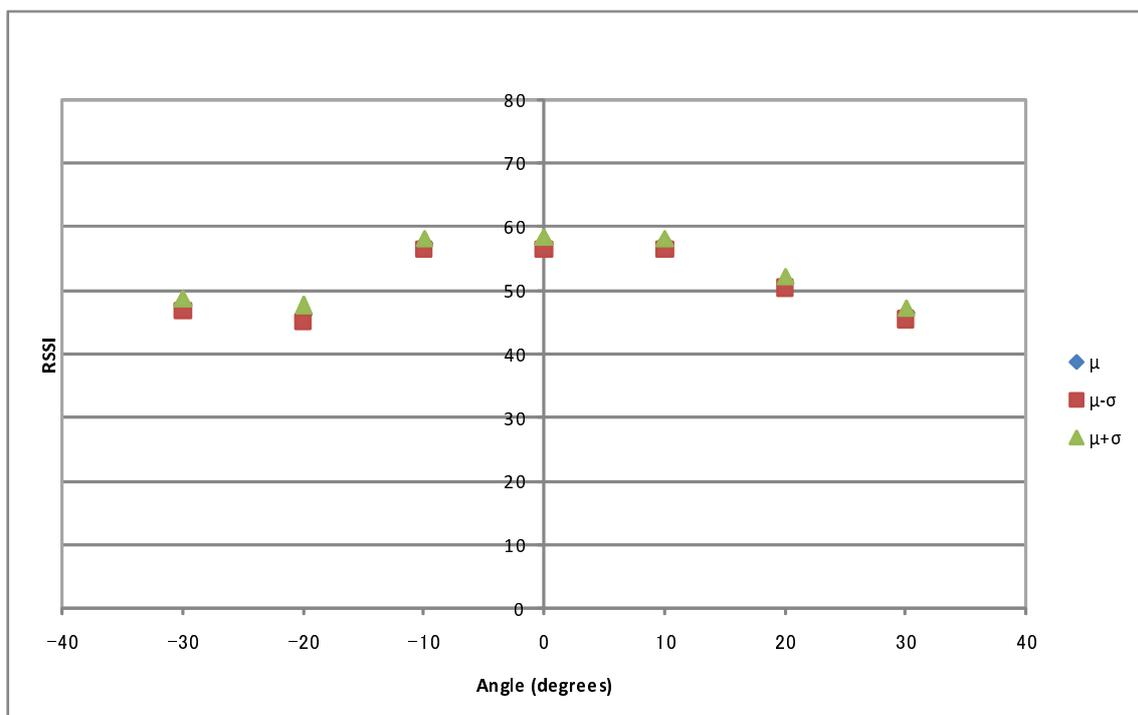
Figure 3.13: RSSI values at 10 degree steps with the antenna 6 meter from signal source (orientation 270 degrees)
