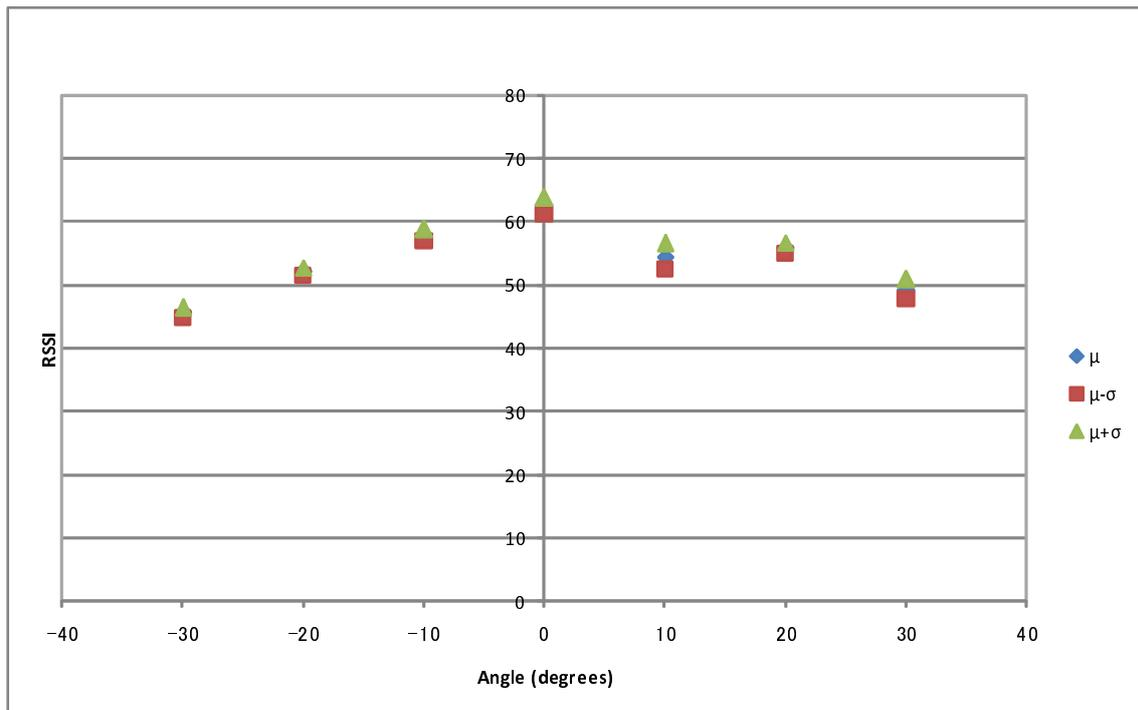
Figure 3.12: RSSI values at 10 degree steps with the antenna 3 meter from signal source (orientation 270 degrees)
