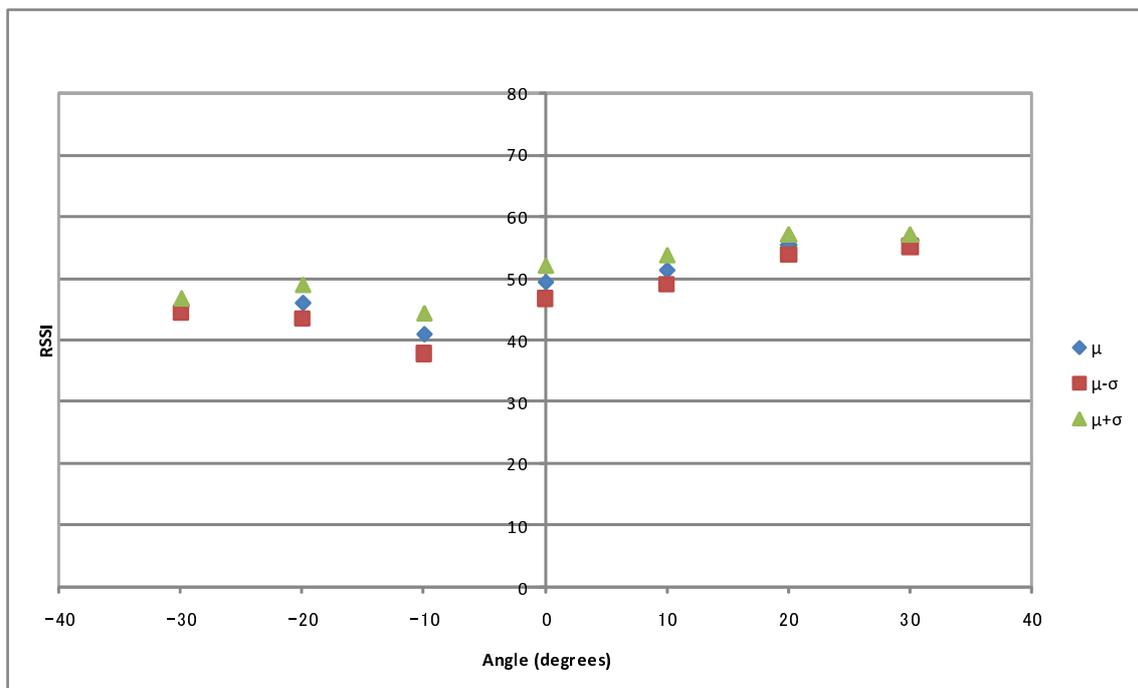
Figure 3.9: RSSI values at 10 degree steps with the antenna 6 meter from signal source
