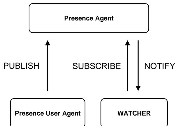
Figure 2.2: Presence messaging mechanism in SIMPLE
