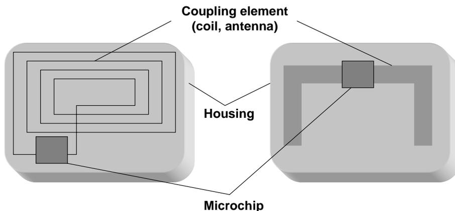
Figure A.2: Two examples RFID transponders (basic layout)(adapted from [2])
