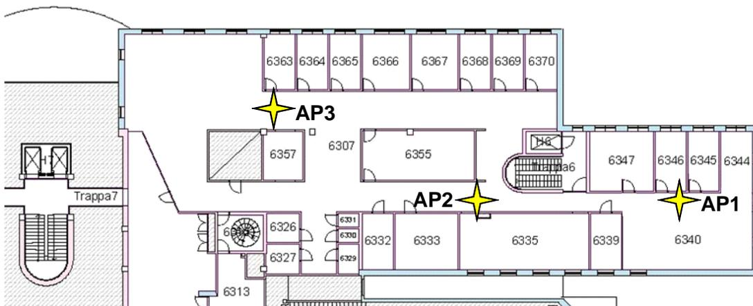
Figure 3.3: Wireless Access Points and the floor plan
