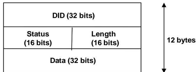
Figure 4.2: Data structure of prism monitoring header item
