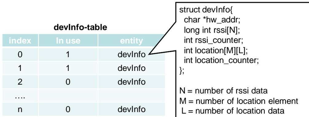
Figure 4.5: Data structure used to store the device information
