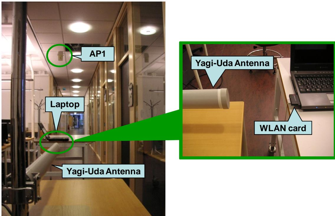
Figure 3.2: Antenna pointed towards the exit door and the laptop on a cart.
