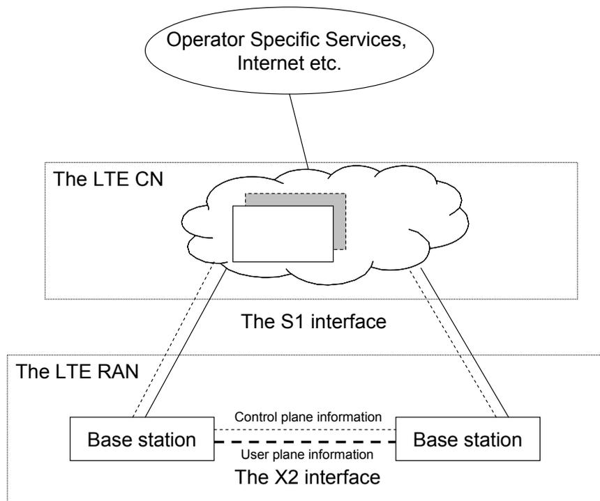
**Figure 6: A simplified model of the LTE architecture**
