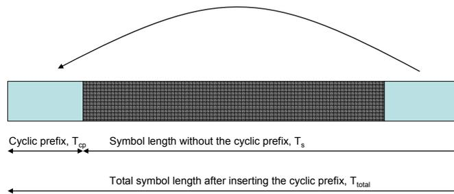
**Figure 4: Adding a cyclic prefix to an OFDM symbol**
