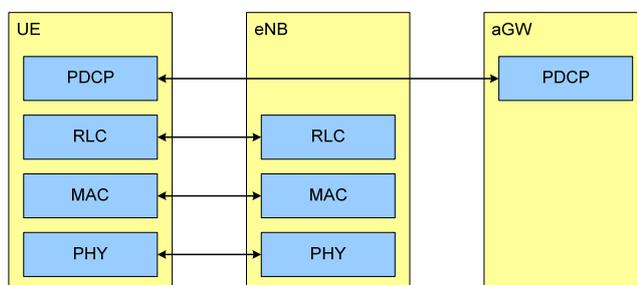
**Figure 8: User plane architecture for LTE [41]**
