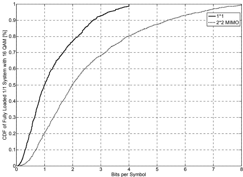
Figure 14: CDFs of the LTE System Model (Normal Cyclic Prefix)
