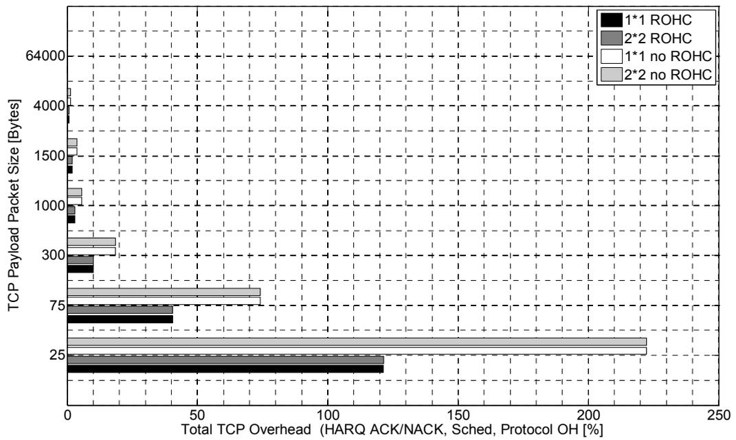
**Figure 27: Total Payload Overhead per TCP Paket**
