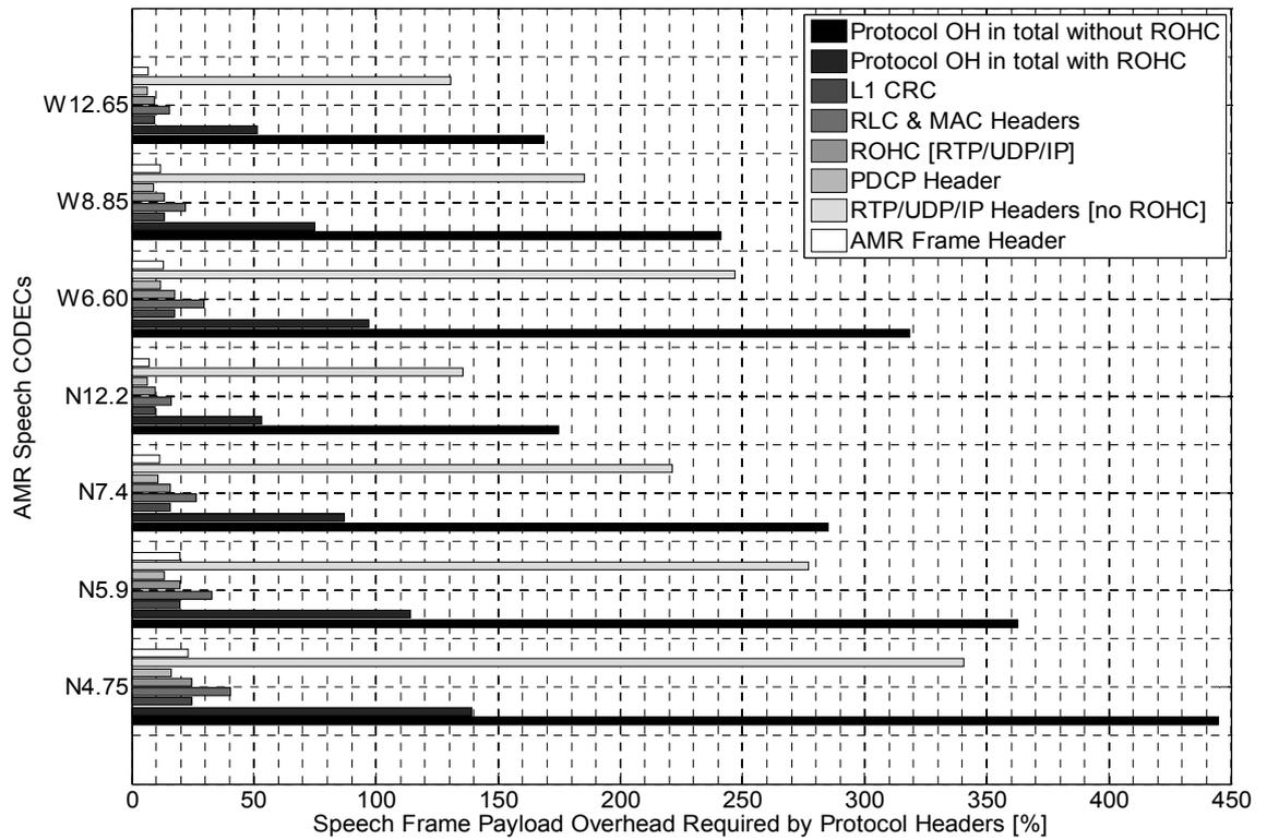
**Figure 22: Protocol overhead for AMR packets**
