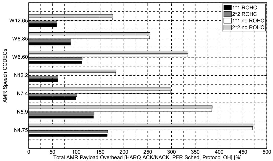
**Figure 26: Total Payload Overhead per AMR Speech Frame (Persistent Scheduling)**
