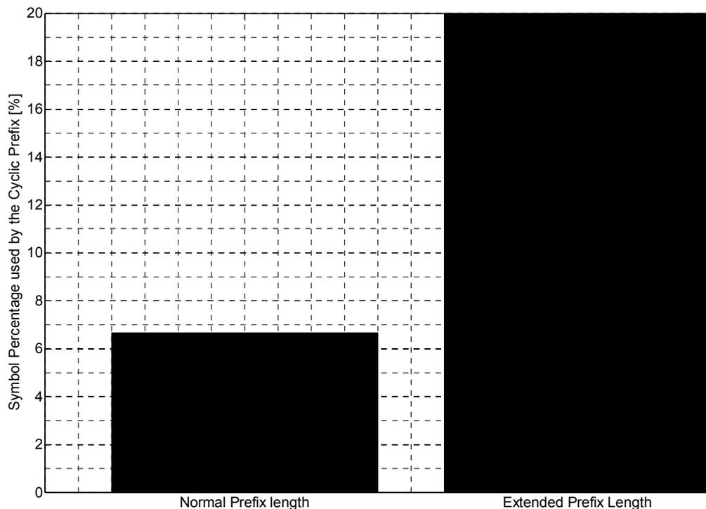
**Figure 16: Cyclic Prefix Overhead per Symbol**
