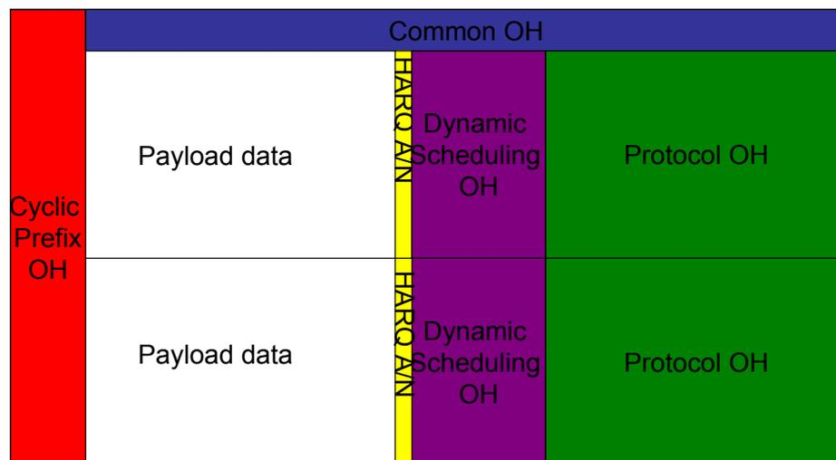
**Figure 15: A Schematic Overhead Constellation in LTE for an AMR 12.2 CODEC using the Normal Cyclic Prefix**
