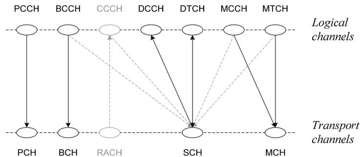
**Figure 13: Suggested mapping between logical channels and transport channels [35]**
