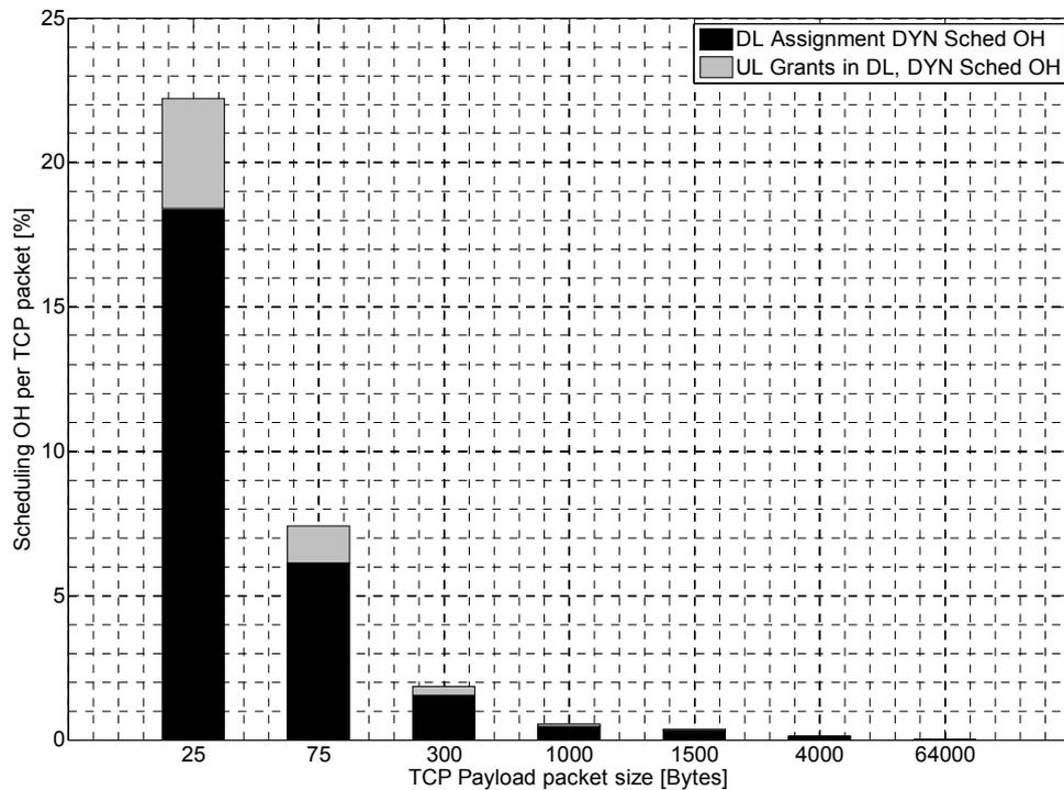
**Figure 21: Scheduling Overhead for TCP packets**
