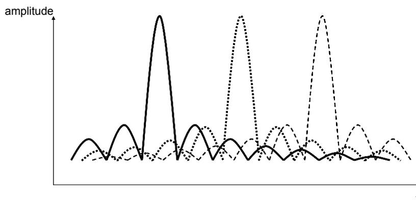
**Figure 1: Three FDM carriers separated by guard bands**
