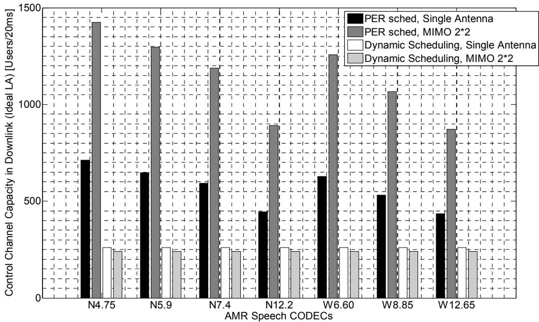
**Figure 30: Estimated Control Channel Capacity**
