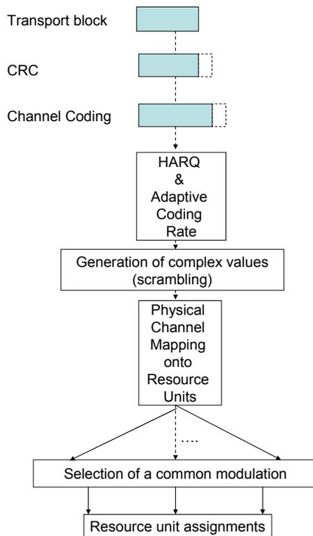
**Figure 12: Basic Modulation and coding of Resource blocks [27]**
