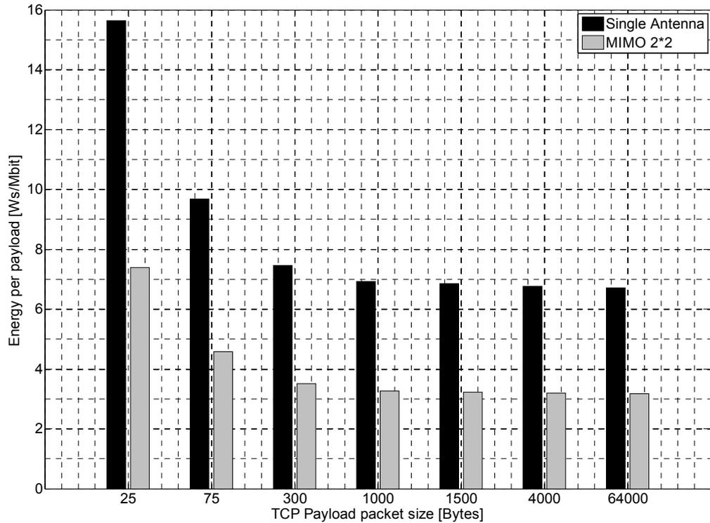
Figure 33: Energy per TCP Payload
