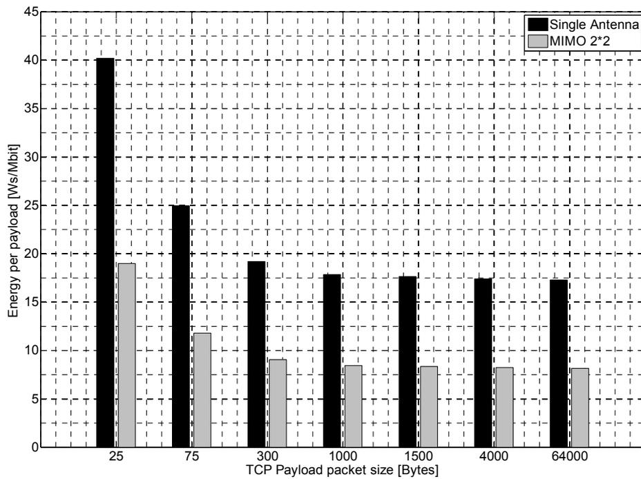
Figure 40: Energy per TCP Payload (extended CP)
