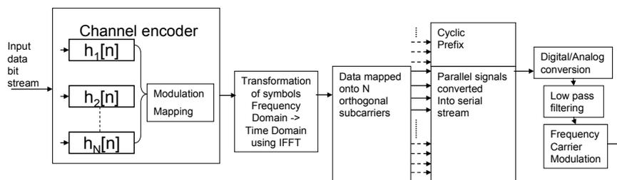
**Figure 2: A simplified model of a downlink OFDM transmission**
