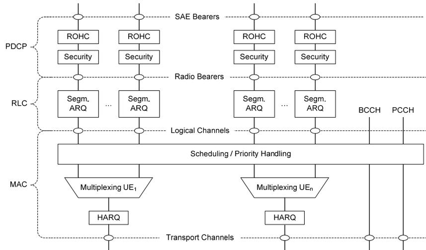
**Figure 9: The Structure for Layer 2 on the downlink [31]**
