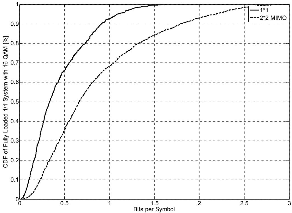
Figure 36: CDFs of the LTE System Model (Extended Cyclic Prefix)
