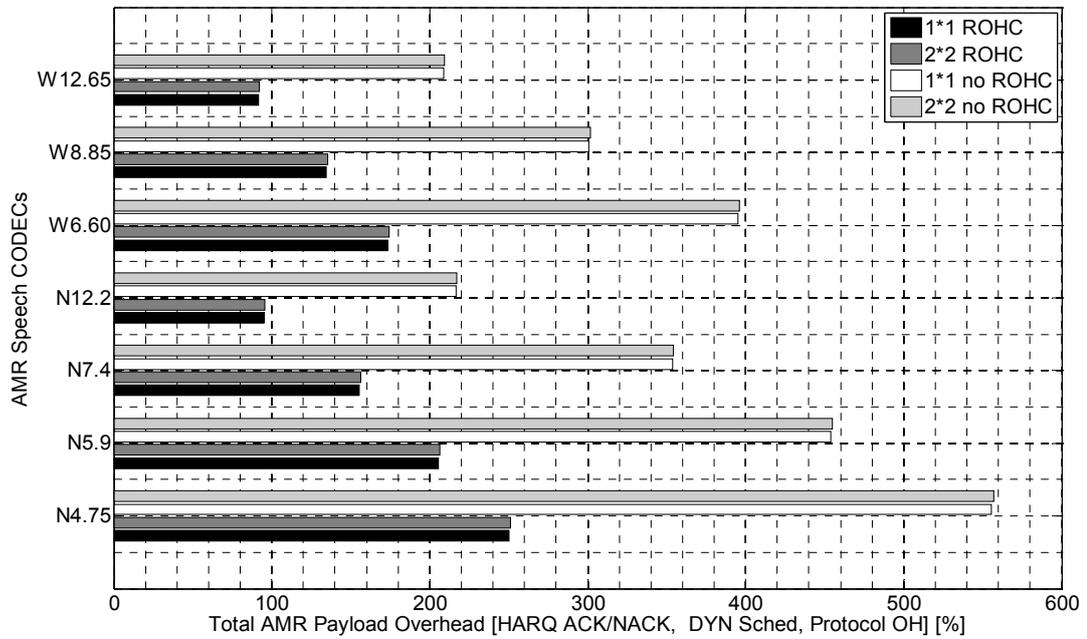
**Figure 25: Summarized Payload Overhead per AMR Speech Frame (Dynamic Scheduling)**
