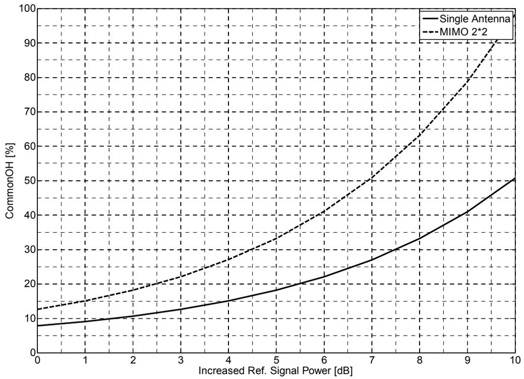
**Figure 35: System Level Control Overhead Impacts from Increased Reference Signal Power**
