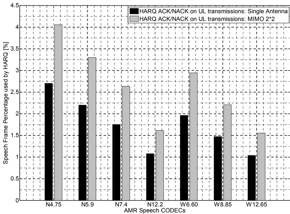
**Figure 19: HARQ ACK/NACK Overhead**
