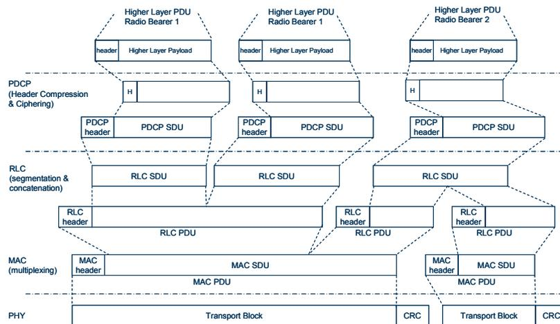
**Figure 10: The flow of user data in a downlink transmission [41], [31]**
