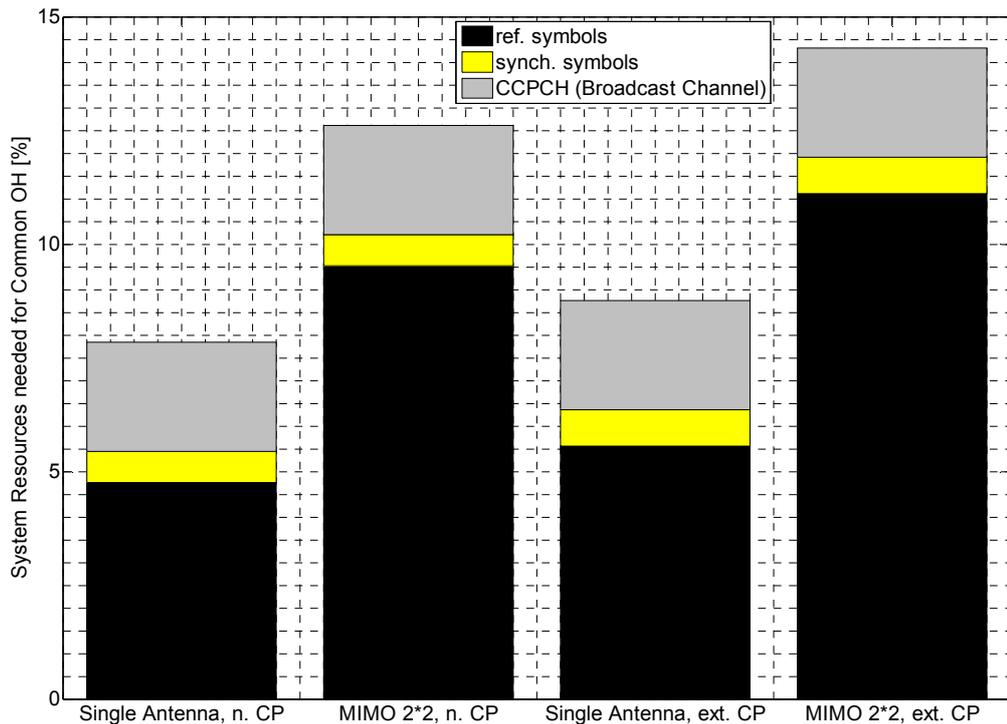
**Figure 17: Common Control Information Overhead for Normal and Extended Cyclic Prefix Length**
