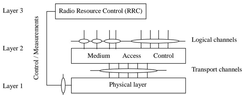
**Figure 7: Radio Interface Protocol Architecture around the physical Layer [30]**
