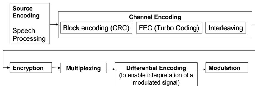
**Figure 3: Basic elements of a transmission chain on the physical layer**
