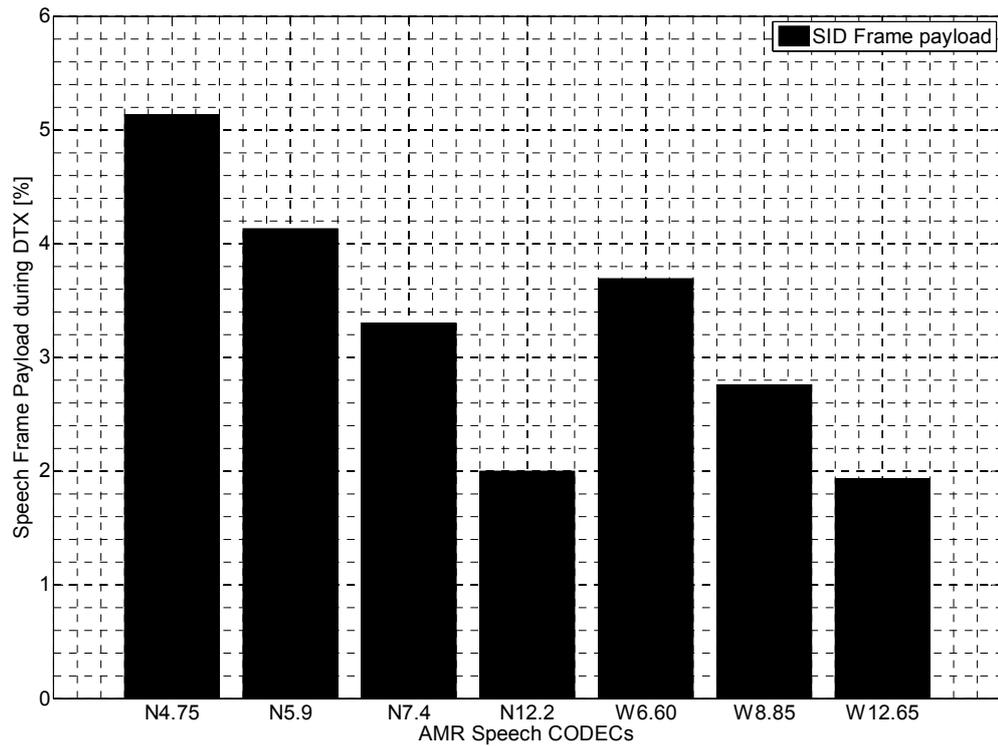
**Figure 18: AMR Payload transmitted during DTX periods**
