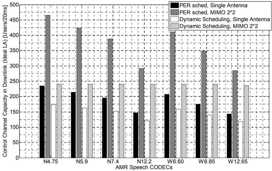
**Figure 37: Estimated Control Channel Capacity (extended CP)**
