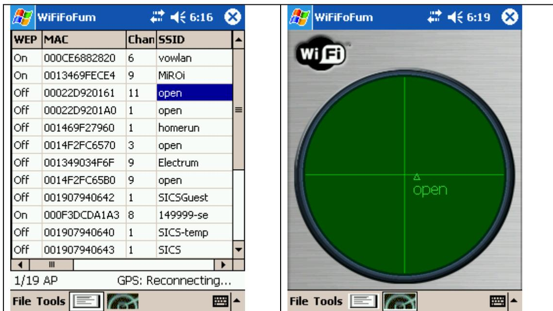
**Figure 6. WiFiFoFum. Radar view conveys distance to access points.**
