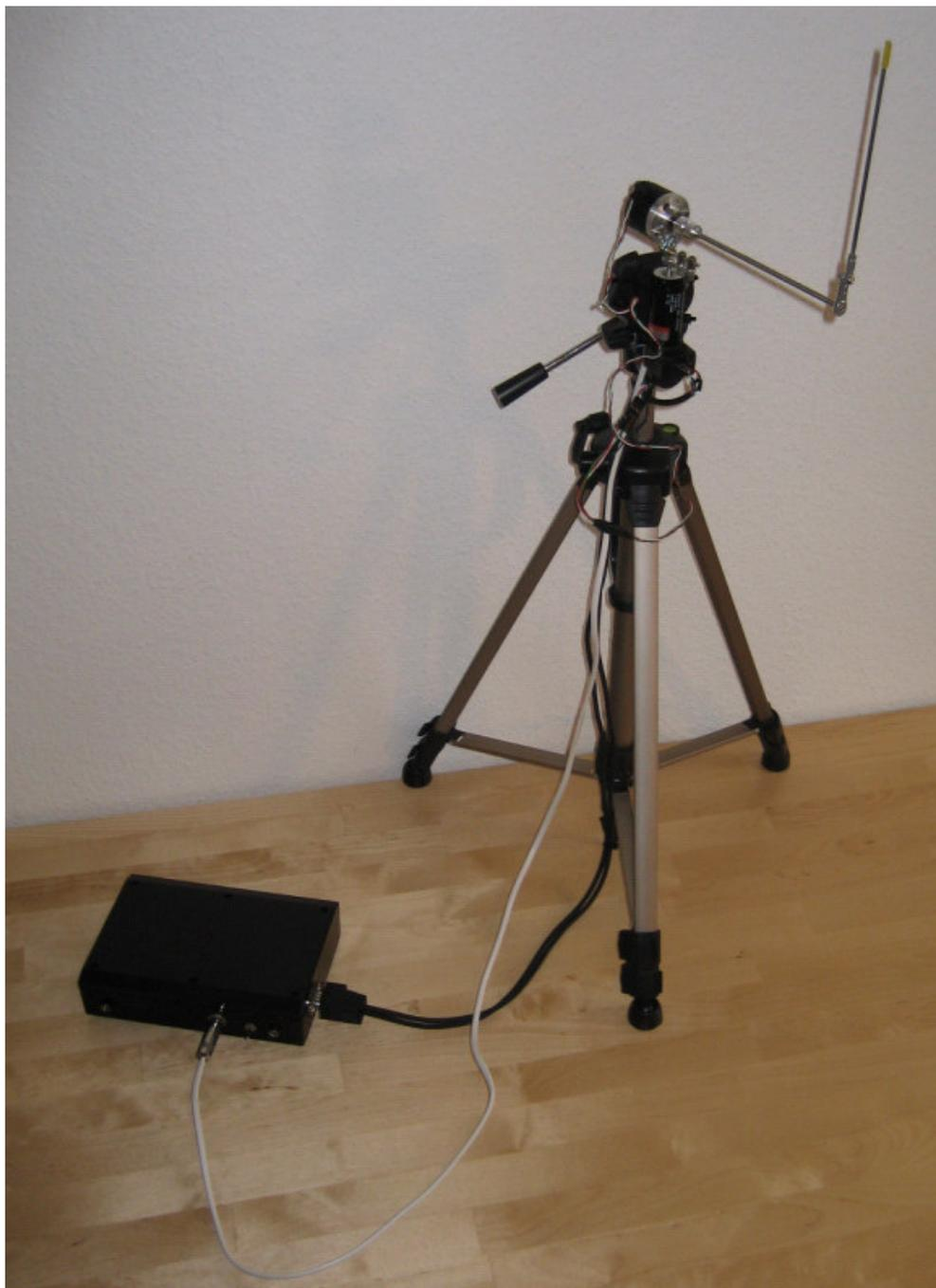
The inverted pendulum and the pendulum interface box
