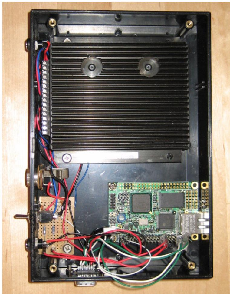
**Inside of the pendulum interface box**
