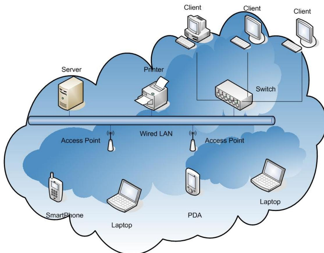
Figure 10: WLAN using multiple access points
