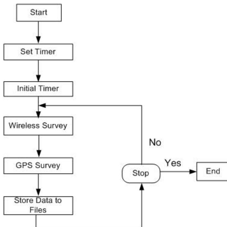
Figure 13: Data flow of Survey Application
