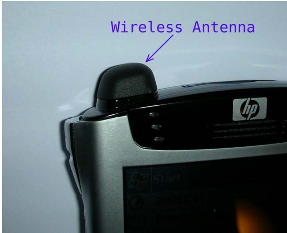
Figure 12: Cover for WLAN antenna on the iPAQ
