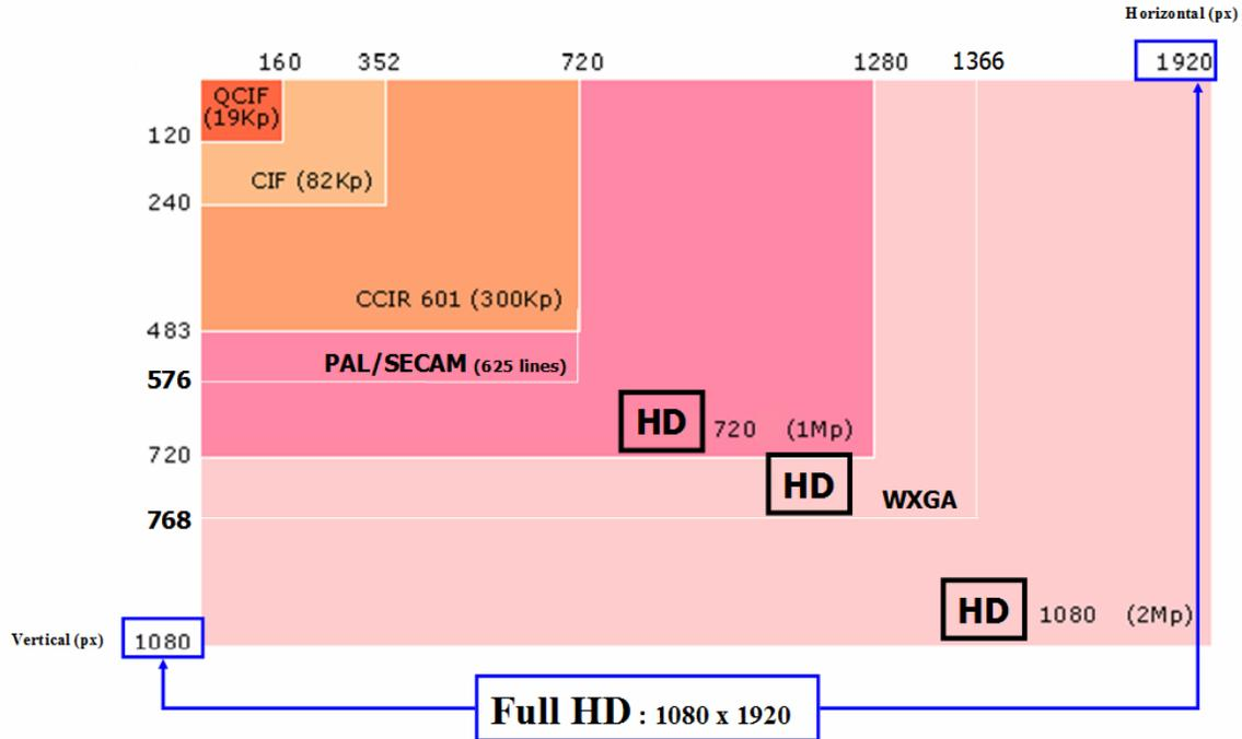
While the Standard Definition PAL has 576 lines (625 lines for French SECAM), two main image resolutions currently exist for HD, as shown in Figure B.2: 768 and 1080 lines.
