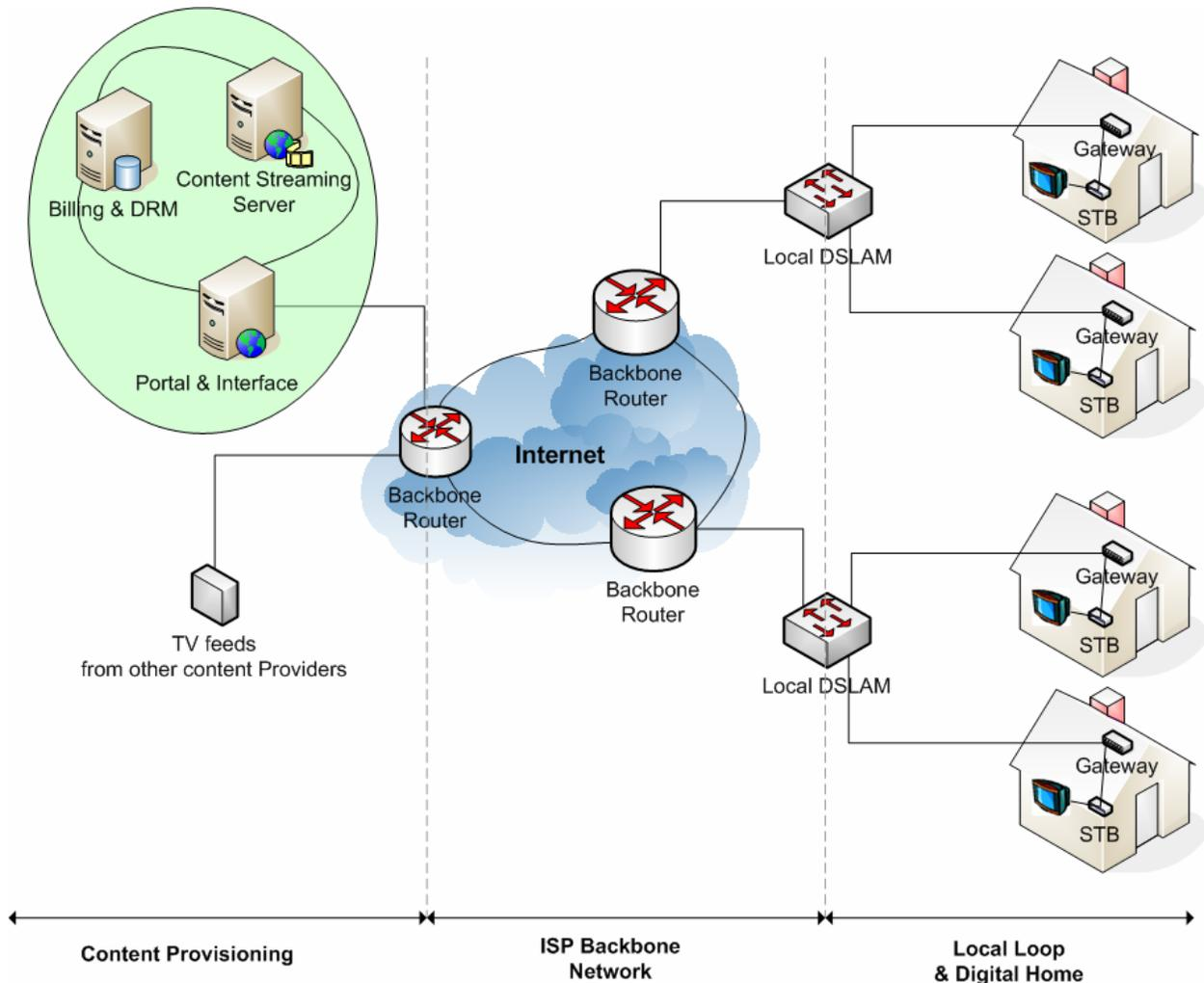
Figure B.5 IP TV network architecture<sup>130</sup>
