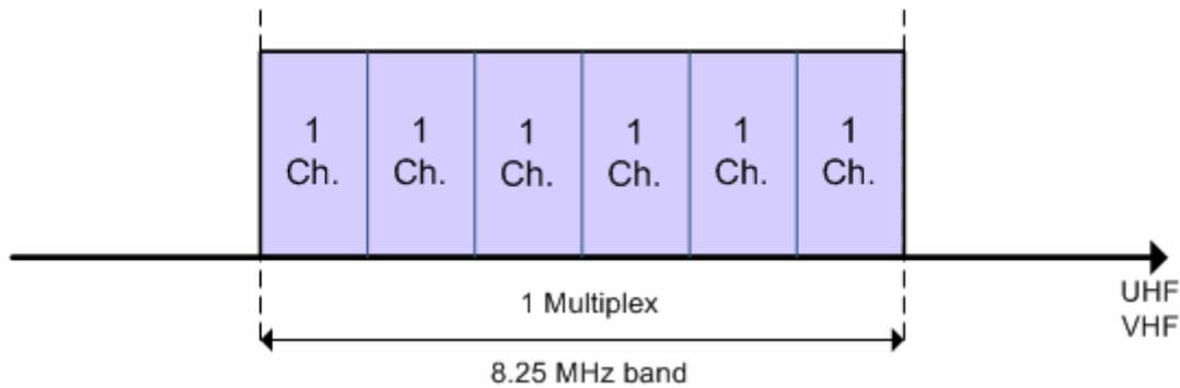
**Figure 4.1 Digital multiplexing structure**
