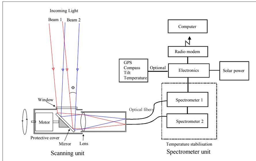
Figure 1-4 Schematic view of the Double Beam Scanning mini-DOAS instrument [18]
