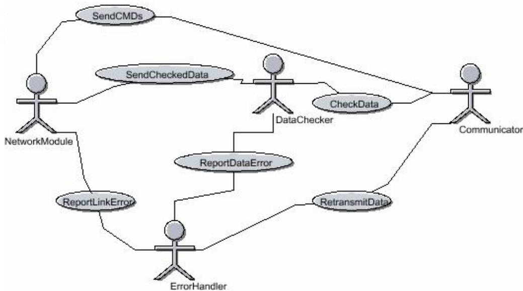
Figure 3-4 Link module of basestation
