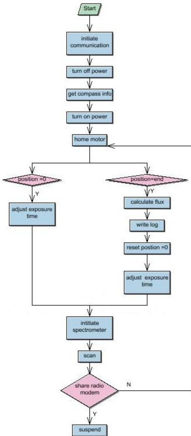
Figure 4-3 Flow chart of the remote control program
