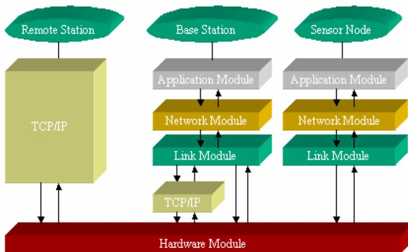
Figure 3-1 Module structure
