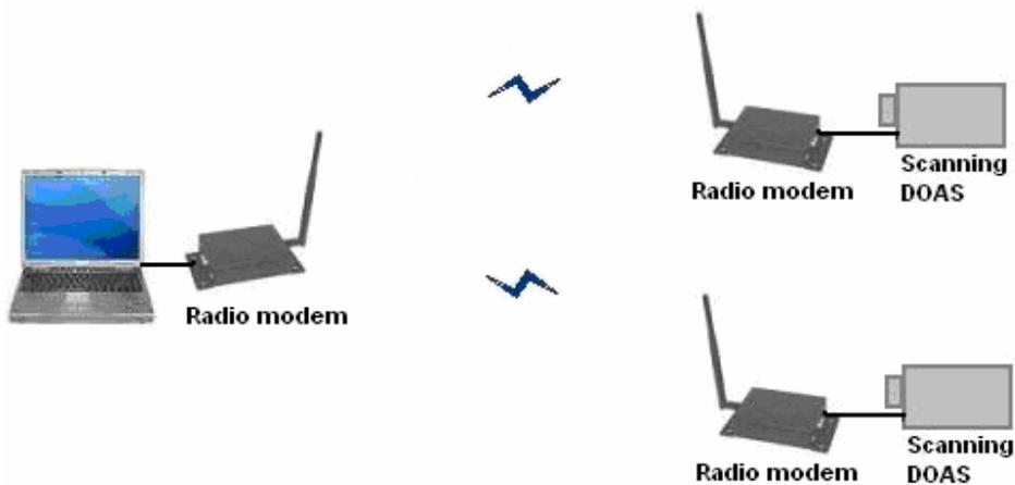
Figure 4-2 Radio network solution for volcano monitoring sensor network
