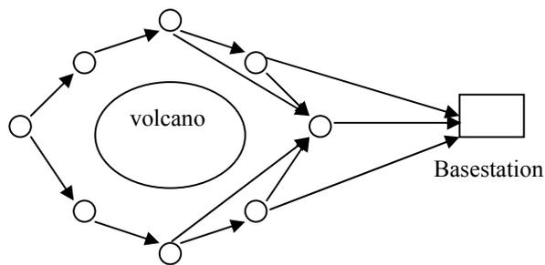
Figure 2-5 An example topology for a volcano sensor network
