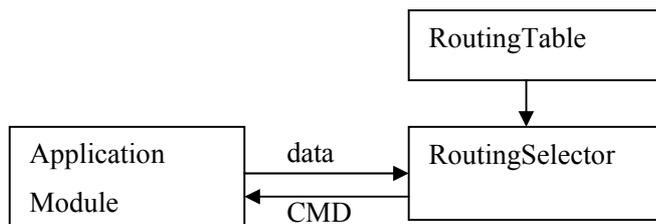
Figure 3-6 Network module in sensor node
