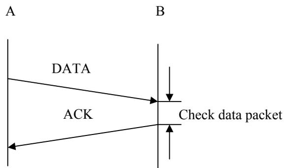
Figure 2-8 (a) Error control in data link layer - normal communication
