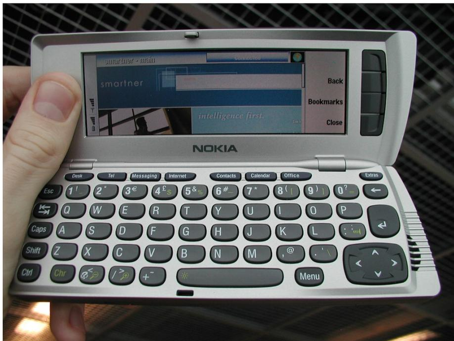
Figure 2.8: The Nokia 9210 Communicator with EPOC OS
