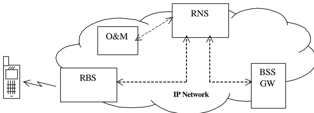
**Figure 2 - 1: Illustrating the different nodes of the complete IP-BSS system. The separate parts are developed by different units within Ericsson, in parallel. The main focus of this project is the verification of functionality in the Radio network Server (RNS) node.**
