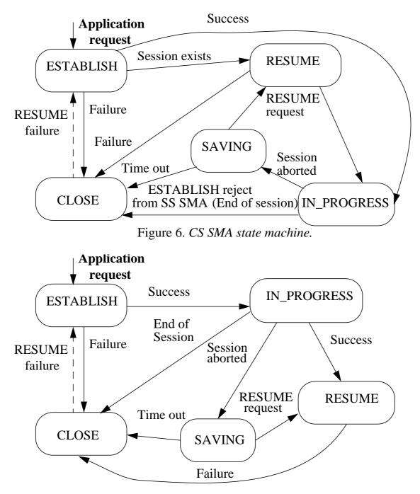
Figure 7. SS SMA state machine.
