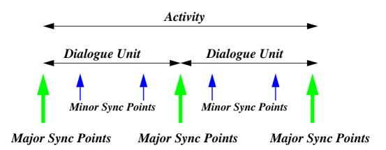
Figure 2. Types of synchronization points.
