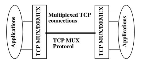
Figure 11. TCP multiplexer architecture.
