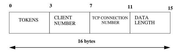
Figure 13. TCP mux header.
