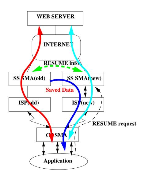
Figure 9. Scenario with one SS SMA per ISP.
