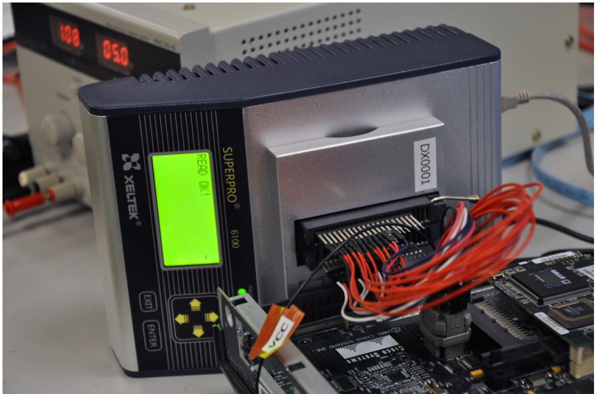
Figure 4-13: Programmer connected to CISCO1712 NVRAM chip.
